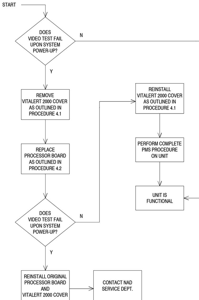
GUIDE 3: FIRMWARE TEST fails upon system power-up
