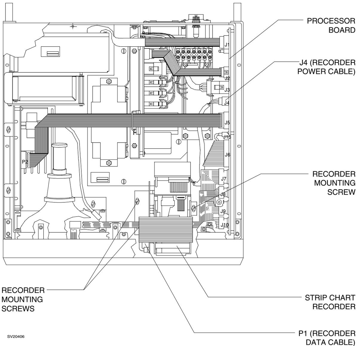
Figure 4-6: REPLACEMENT OF STRIP CHART RECORDER
