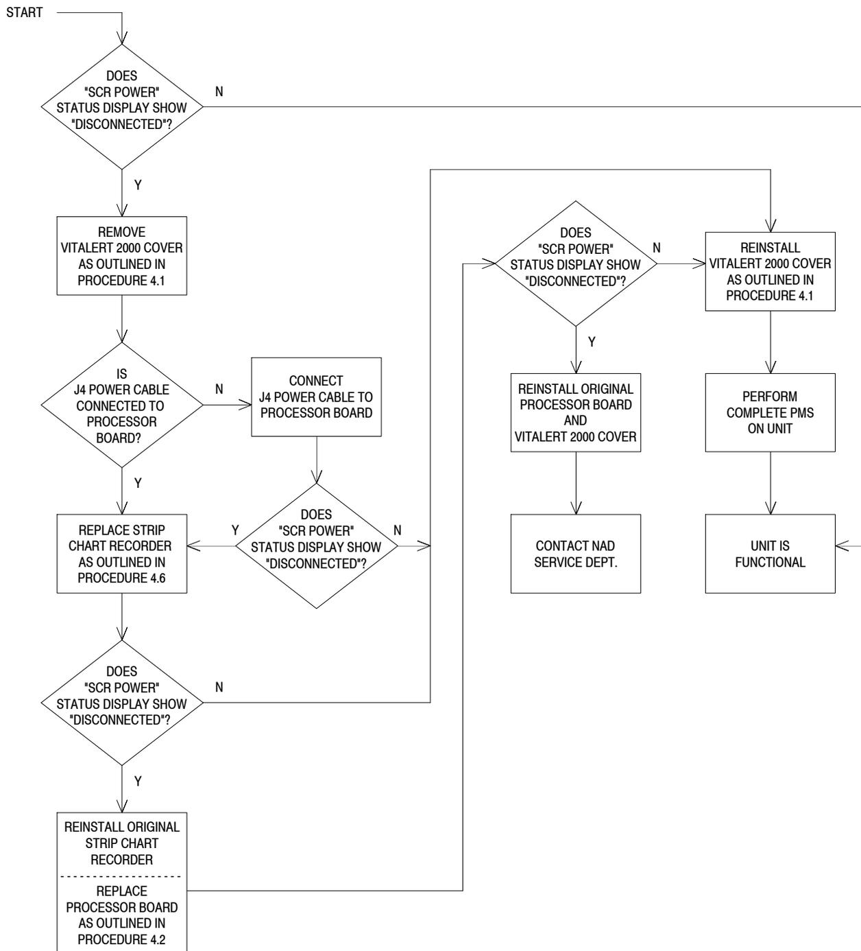
**GUIDE 27: SCR DATA status is DISCONNECTED**
