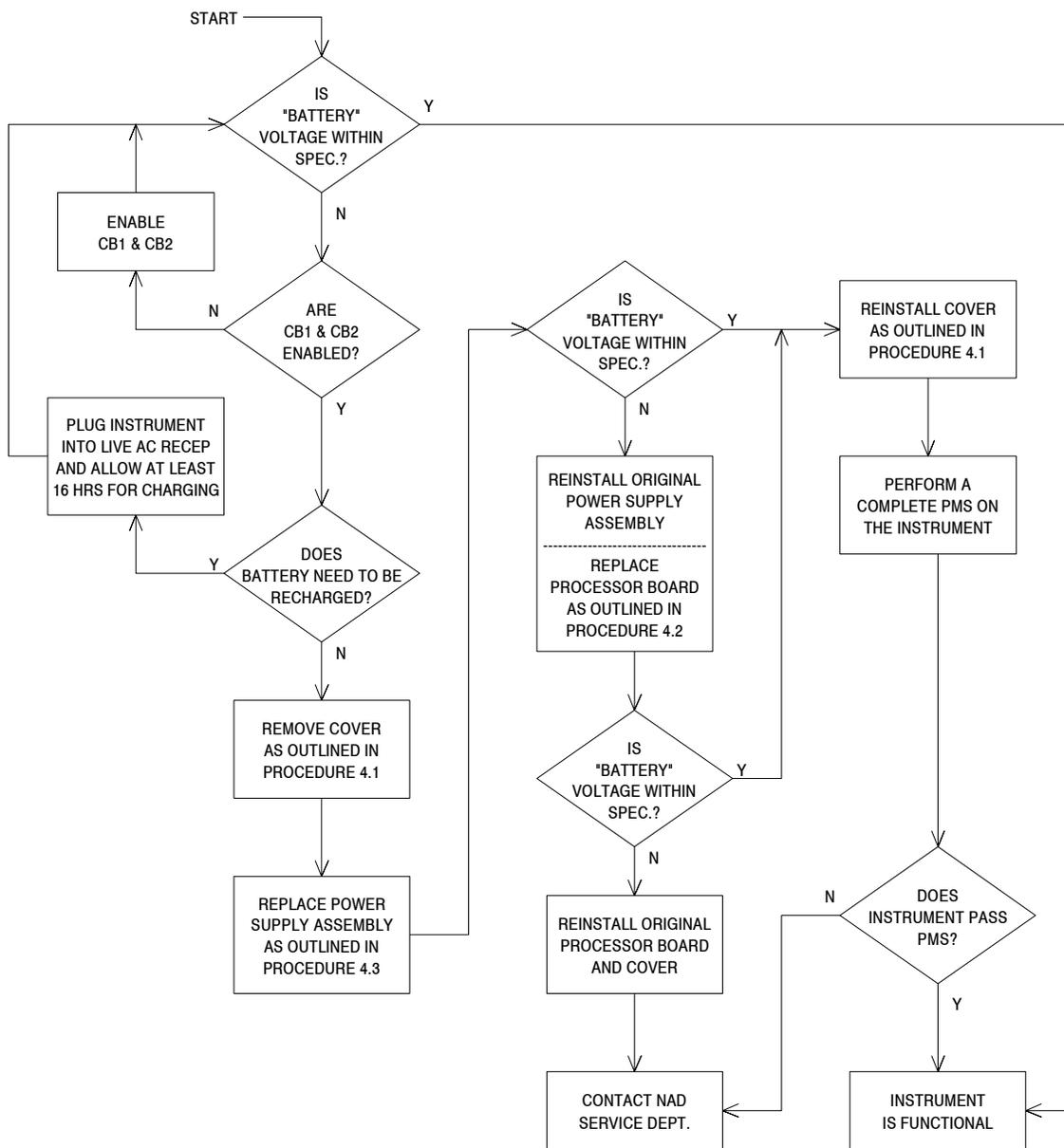
**GUIDE 15: CB BATTERY voltage is not within specifications**
