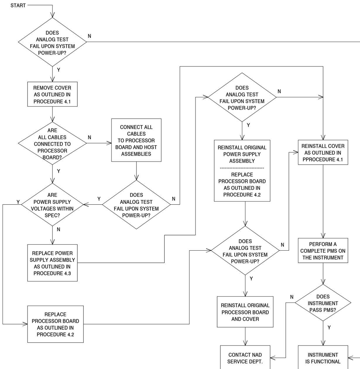
GUIDE 7: AUDIO TEST - PRIMARY or BACKUP fails upon system power-up
