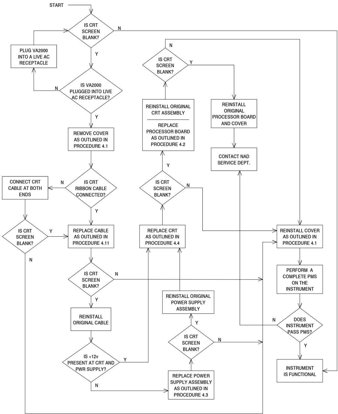
GUIDE 2: VIDEO TEST fails upon system power-up
