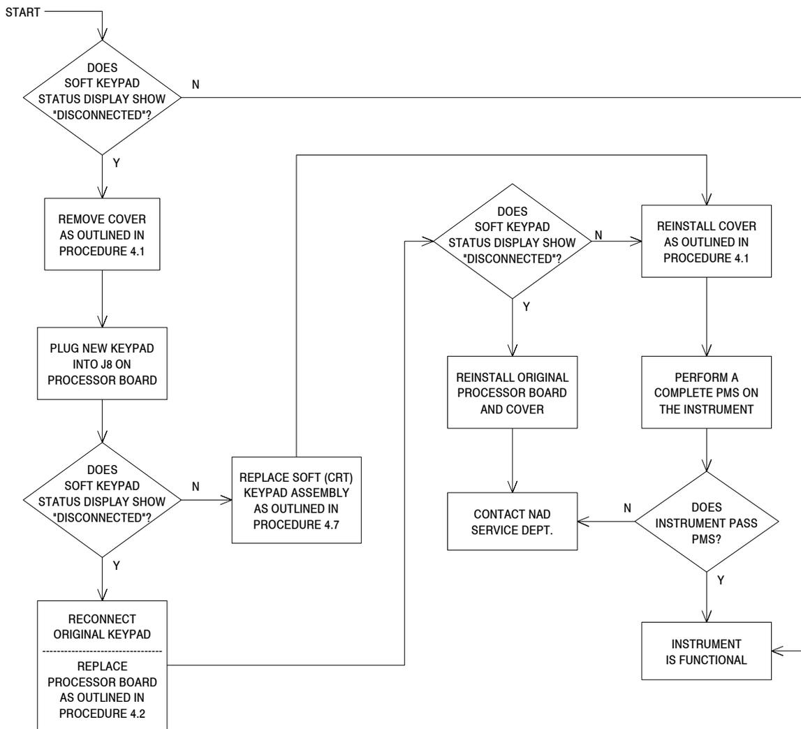
GUIDE 24: ON/STANDBY KEYPAD status is DISCONNECTED
