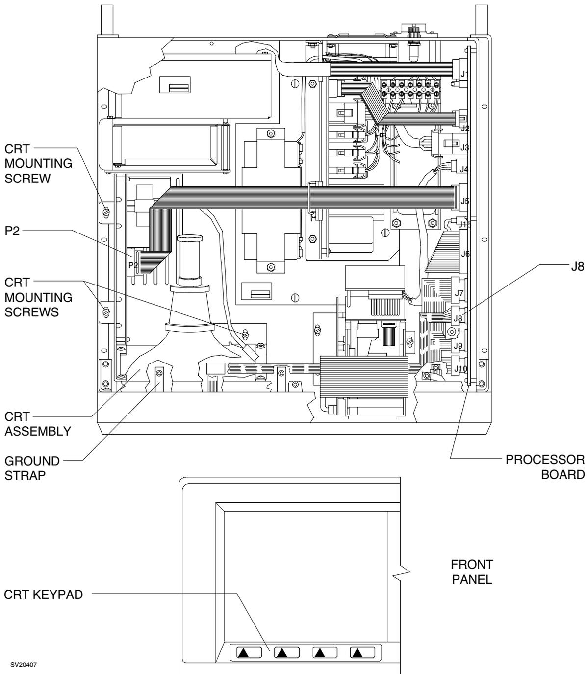
Figure 4-7: REPLACEMENT OF CRT KEYPAD
