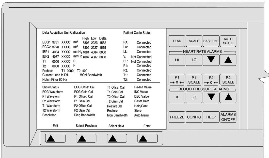
Figure 5-3: DAU MANUAL CALIBRATION SCREEN
