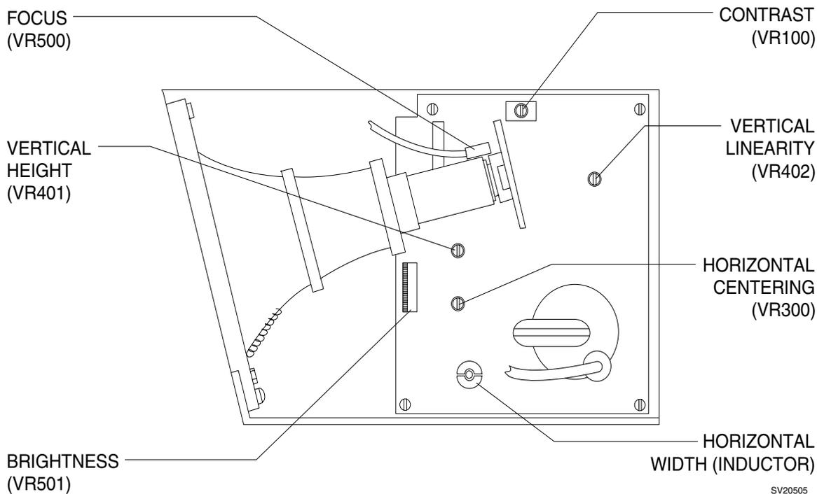
**Figure 5-2: COMPUTRON CRT ADJUSTMENTS**
