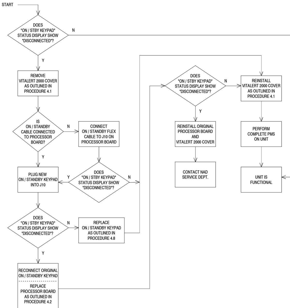
**GUIDE 25: SCR KEYPAD status is DISCONNECTED**
