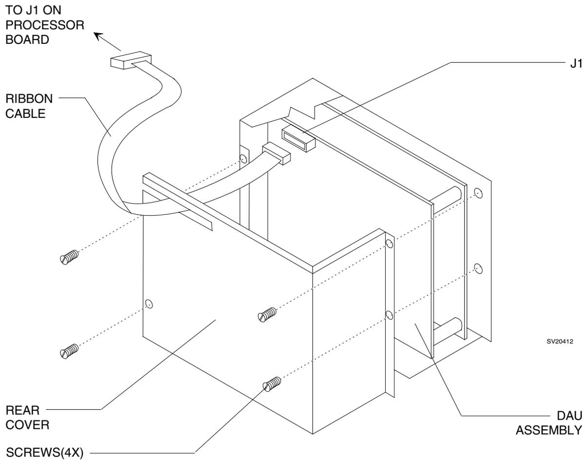
Figure 4-12: REPLACEMENT OF DAU - PROCESSOR BOARD CABLE
