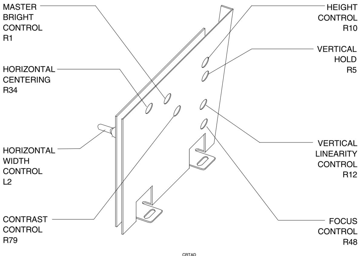
Figure 5-1: WELLS GARDNER CRT ADJUSTMENTS (EARLY MODELS)
