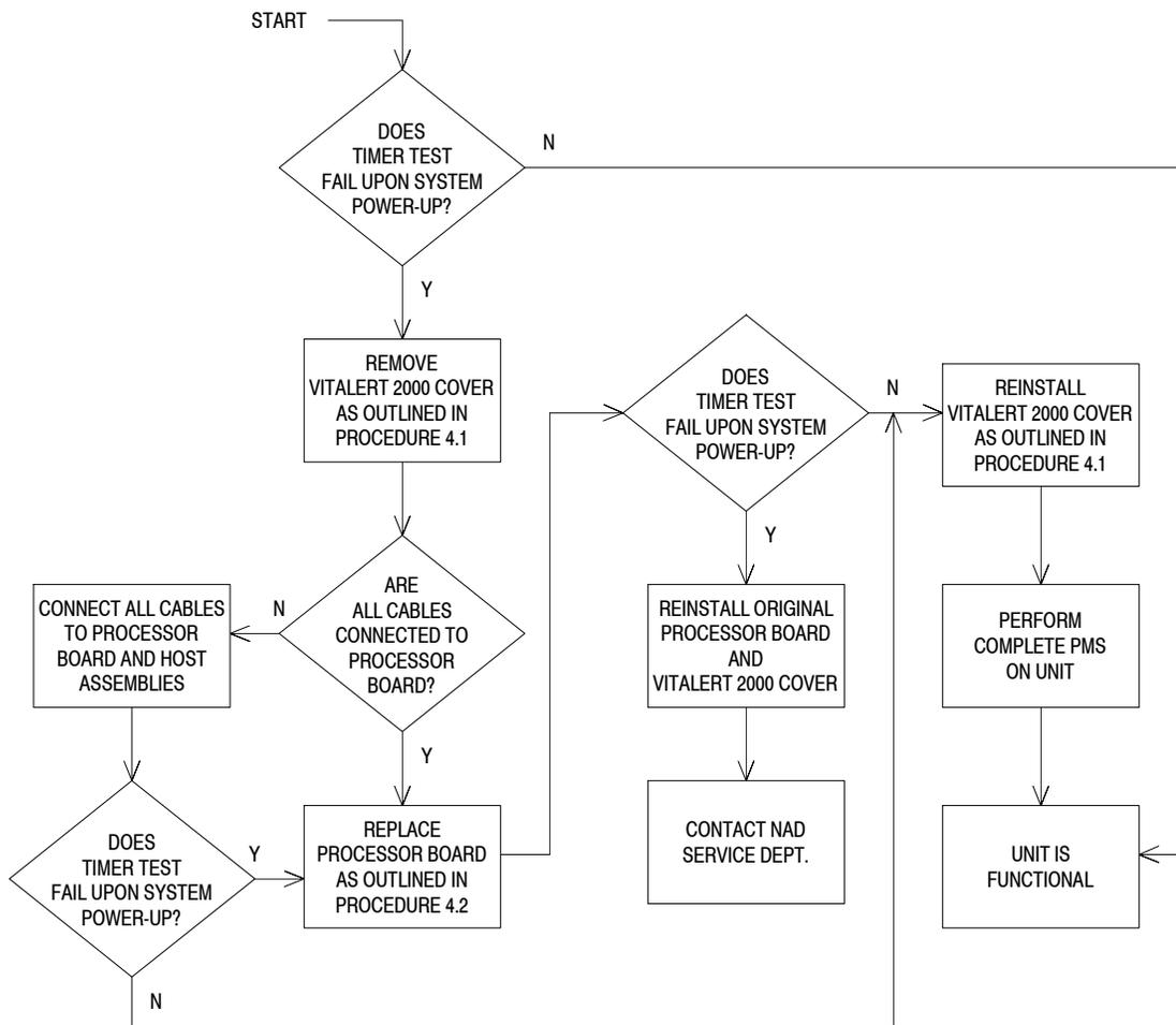
GUIDE 6: ANALOG TEST fails upon system power-up
