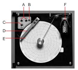
Chart recorder with paper and battery installed.
