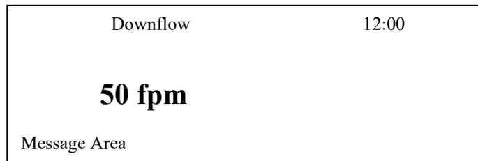
The top line will show the items being displayed along with the time of day. The center of the display will show the downflow velocity value that was entered during the last calibration. The bottom of the display or message area will show active alarms and other status information.
