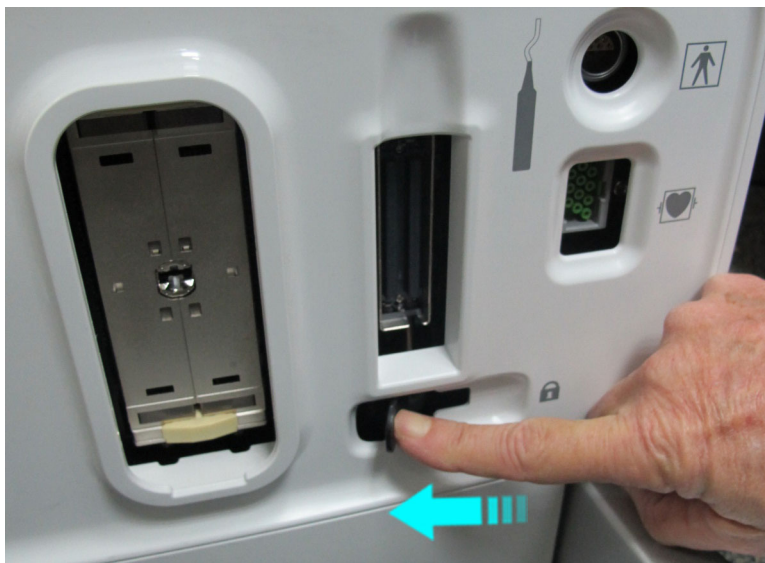
Figure 8-11 RS Probe Connector Lock - OPEN
