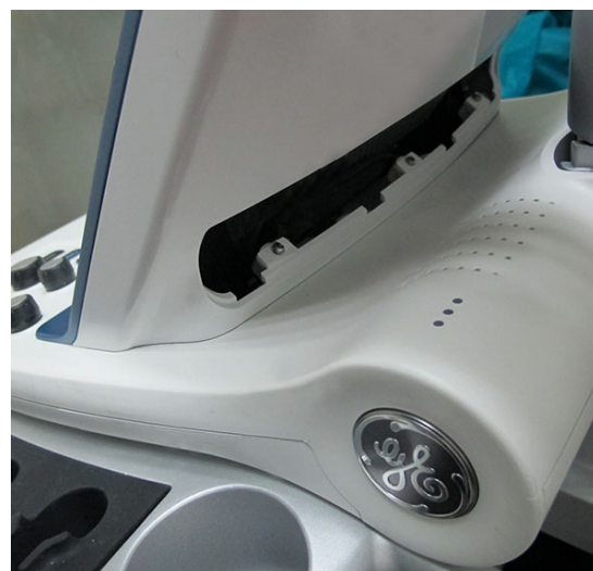
Figure 8-35 Removing the Touch Screen Service Cover
