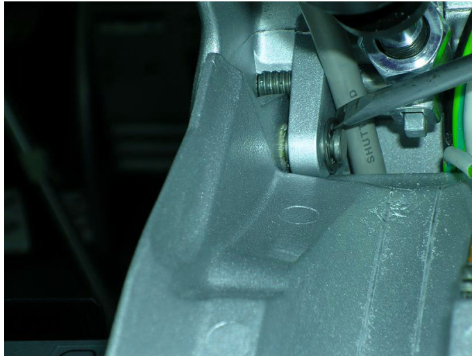
Figure 8-106 Removing Left Securing Clip from Securing Pin
