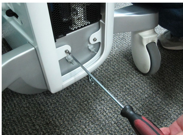
Figure 8-13 Removing Screw from Front Cover Securing Tab
