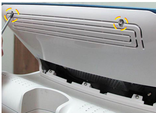
Figure 8-38 Removing the Rear Cover (Top) Securing Screws
