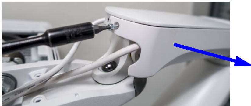
Figure 8-89 Remove the screw and the Upper Service Cover (one side illustrated)
