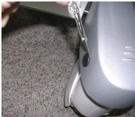
Figure 8-133 Removing the Screw Cap
