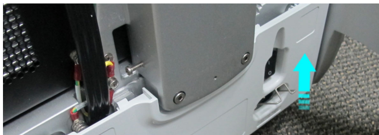
Figure 8-29 Removing the AC Distribution Box Cover
