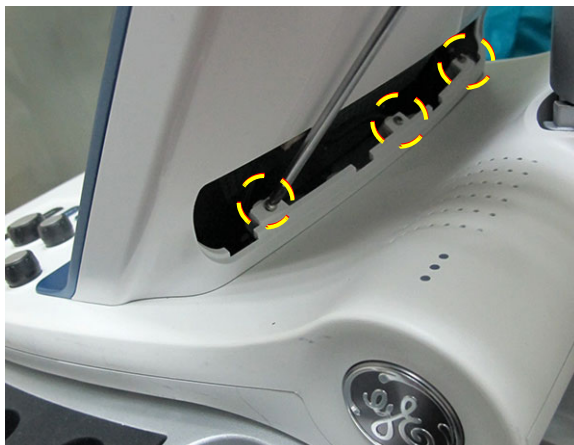
Figure 8-37 Removing the Rear Cover (Base) Securing Screws
