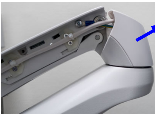
Figure 8-90 Remove the Vertical Service Cover
