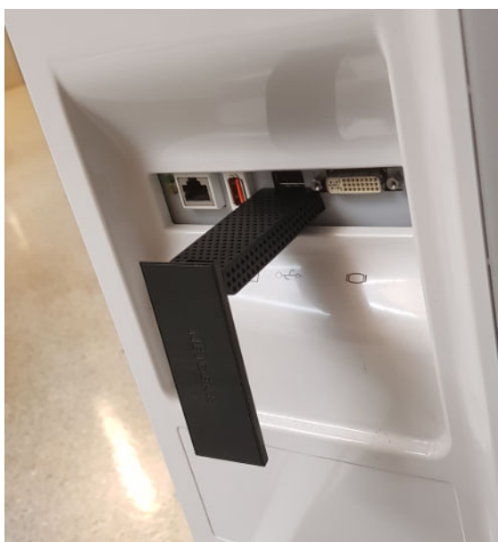
Figure 3-29 Connecting wireless network adapter to rear USB-port
