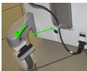
Figure 8-129 AC Power Cable Connected and Routed
