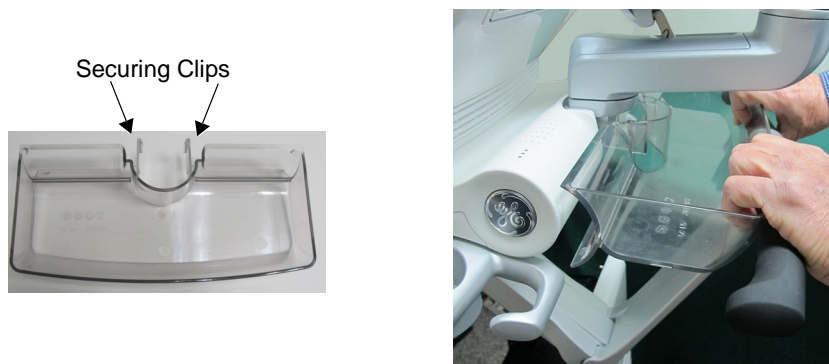
Figure 8-24 Removing the OPIO Basket
