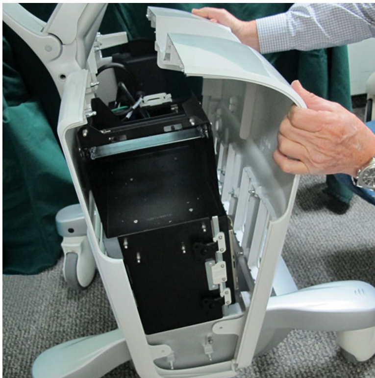
Figure 8-14 Removing the Front Cover
