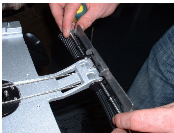
Figure 8-98 Protective Metal Plate Rotated 90 Degrees
