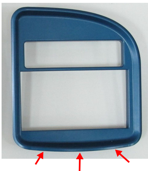
Figure 8-7 Removing the DVD and Printer Cover
