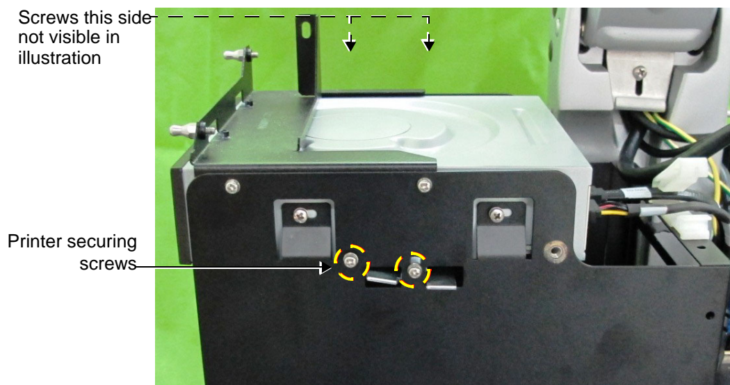
Figure 8-155 Screws Securing Black and White Printer in Compartment
