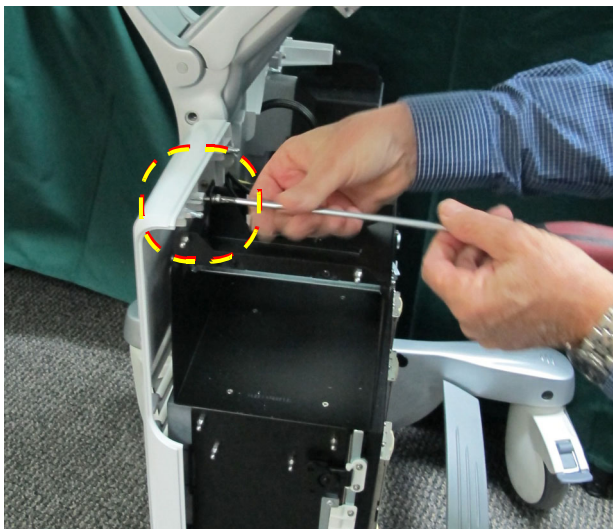
Figure 8-17 Right Rear Cover - Removing Securing Screws
