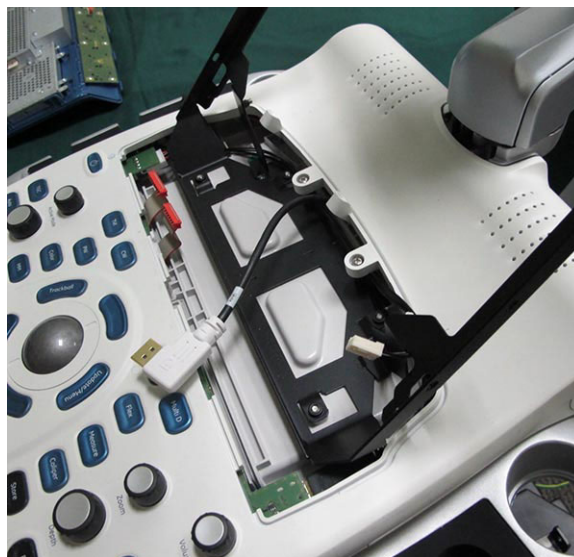
Figure 8-45 Removing the Touch Screen
