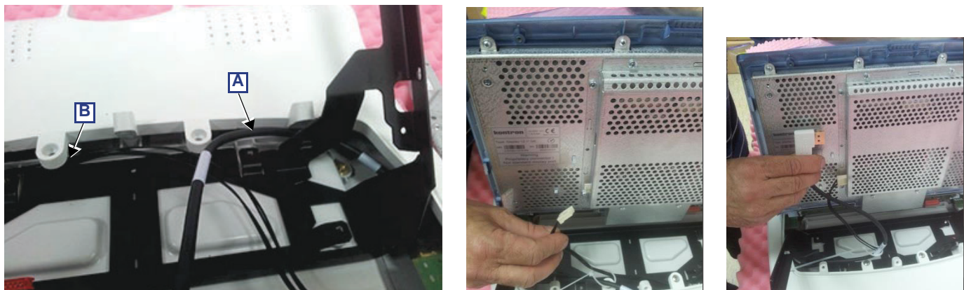
Figure 8-47 Routing and Connecting the Touch Screen Cables
