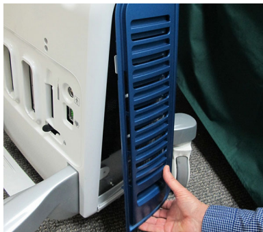
Figure 8-3 Removing the Air Inlet (Left Side) Cover
