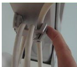
Figure 8-127 Opening the Cable Gate on Probe Cable Holder
