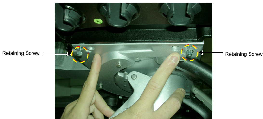
Figure 8-124 Probe Shelf - Viewed from Below indicating Retaining Screws
