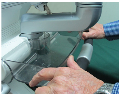
Figure 8-25 Installing the OPIO Basket
