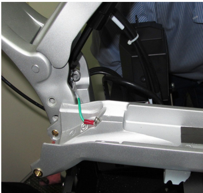
Figure 8-108 Removing the Lower Arm
