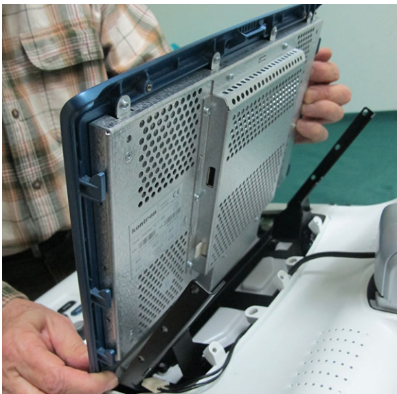
Figure 8-45 Removing the Touch Screen
