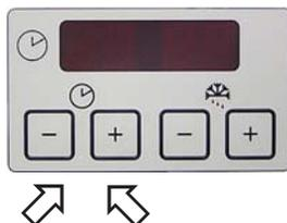
The actual time is set on the panel marked with the clock symbol using the **+** and **-** keys.
