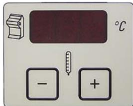
The temperature of the cryochamber is set and indicated on the panel marked with the cryostat symbol.
