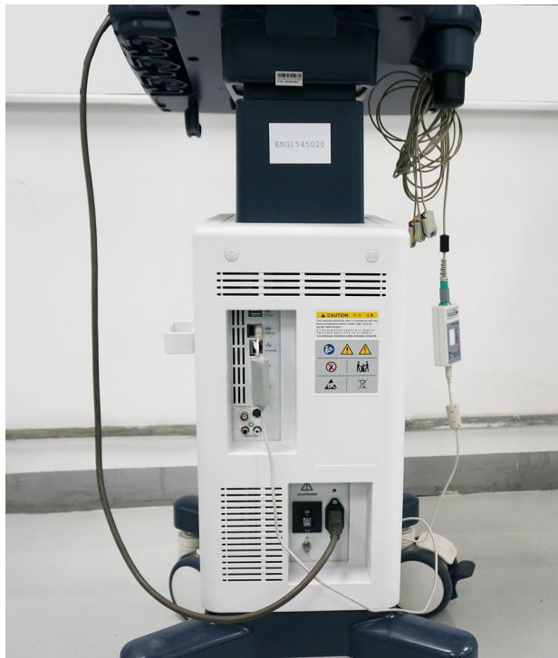
Figure 3-28. Connect ECG to the system
