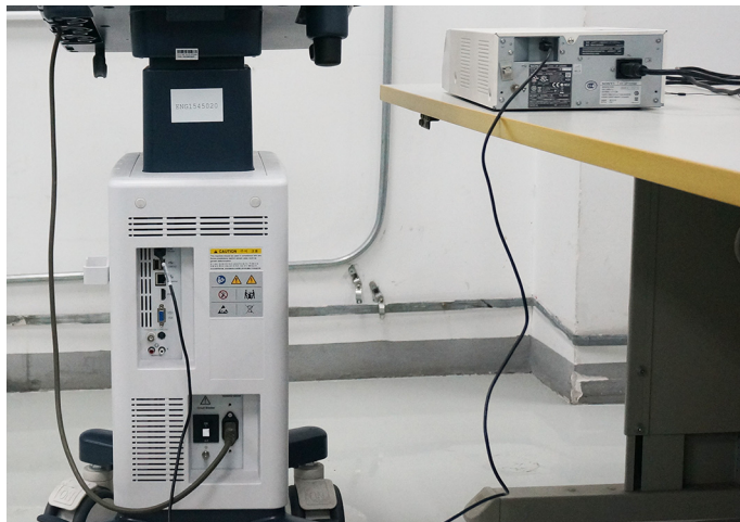
Figure 3-20. Color Printer connection
