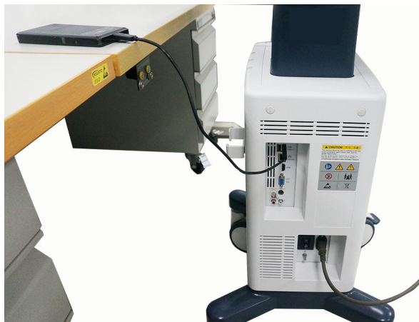
Figure 3-27. Connect HDD to the system
