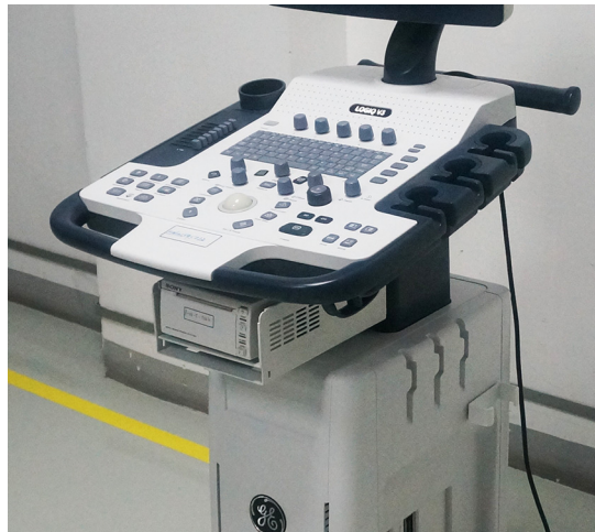
Figure 3-12. Connect UP-D711MD to LOGIQ V3/V5/V5 Expert
