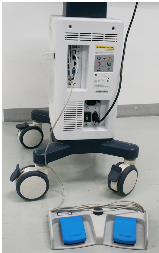
Figure 3-25. Connect Footswitch to the system
