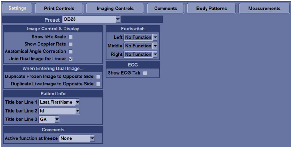
Figure 3-26. Configuring Footswitch Functions
