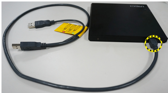
Figure 3-29. Connect Y cable
