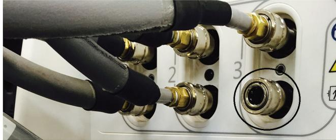
Figure 29: Disconnected hose
