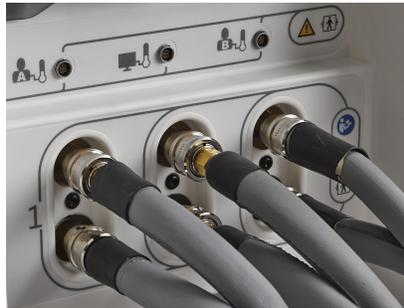
**Figure 25: Hoses connected**
