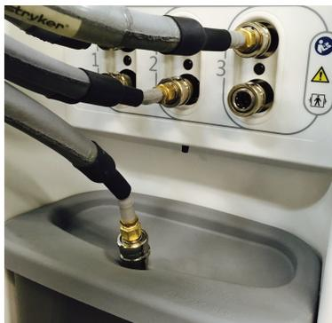
**Figure 32: Bottom hose end in the lid of the reservoir**
