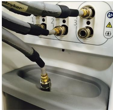
Figure 30: Bottom hose end in the lid of the reservoir
