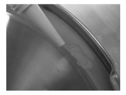
Allow the silicone to set for about 30 minutes. It should be slightly tacky. Close the door of the autoclave or sterilizer. The door will press the silicone into the defect. Excess silicone ensures formation of a seal. Do not remove excess.
