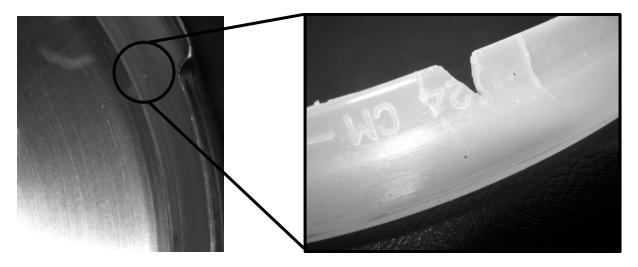
Squeeze a small amount of silicone into the defect. Use excess silicone to fill the defect. Do not scrape off excess silicone.
