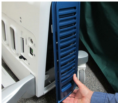
Figure 8-3 Removing the Air Inlet (Left Side) Cover
