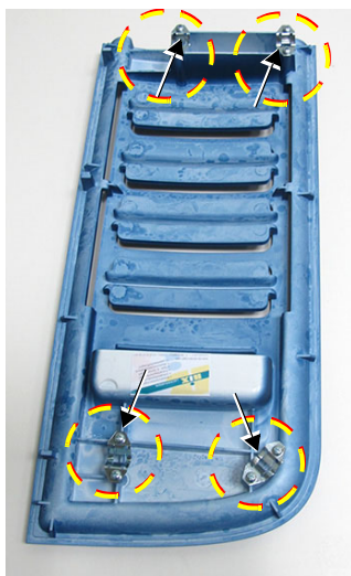
Figure 8-5 Removing the Right Side Cover
