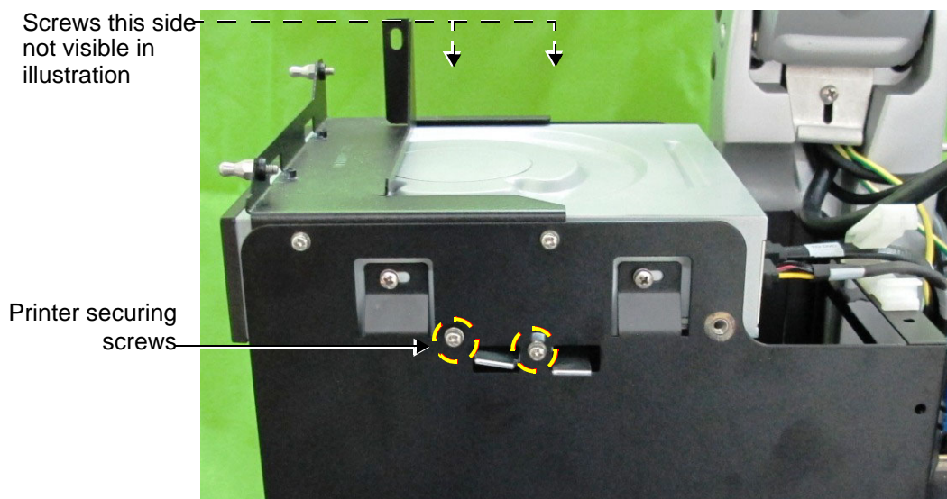
Figure 8-171 Screws Securing Black and White Printer in Compartment
