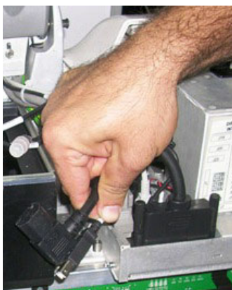
Figure 8-172 Cables Disconnected from Rear of Black and White Printer
