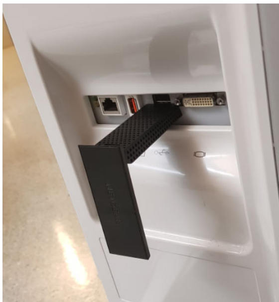
Figure 3-28 Connecting wireless network adapter to rear USB-port
