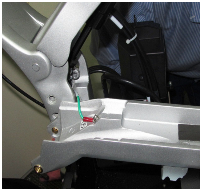
Figure 8-108 Removing the Lower Arm
