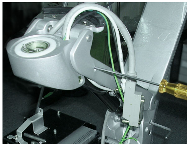
Figure 8-113 Supporting the Upper Gas Spring Bracket with a Screwdriver
