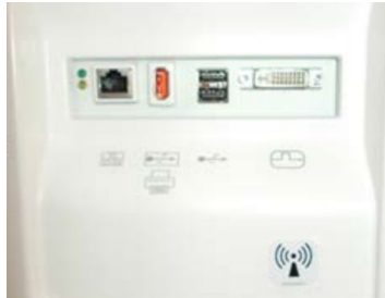
Figure 3-29 Placement of wireless network Label on Vivid S60N/Vivid S70N
