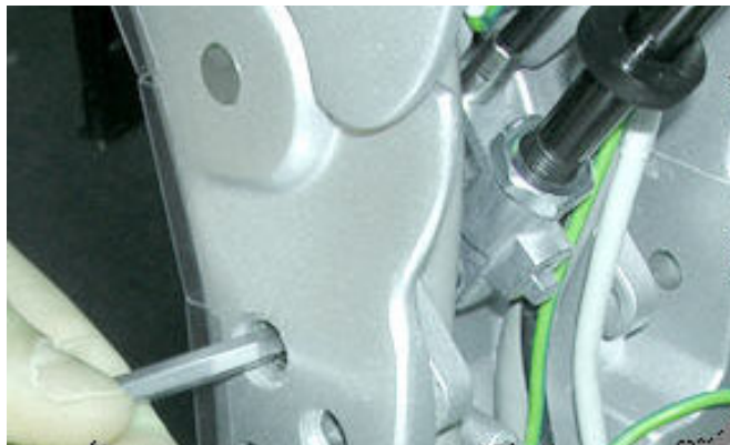
Figure 8-111 Releasing the Securing Screws on Either Side of the Support Arm
