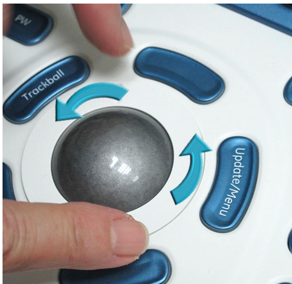
Figure 8-64 Removing the Mechanical Trackball Ring
