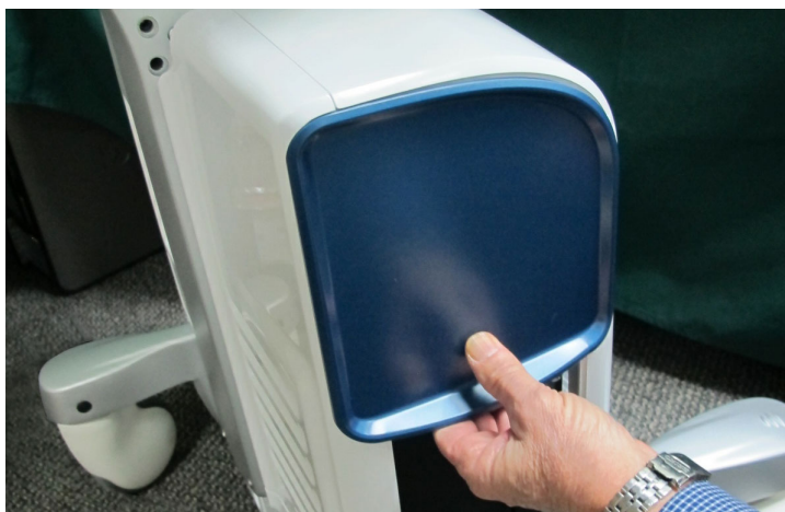
Figure 8-8 Removing the Blank Cover
