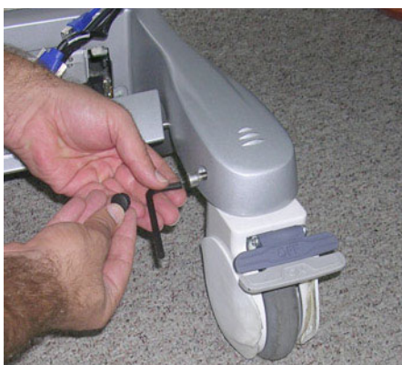
Figure 8-134 Removing the Securing Screw
