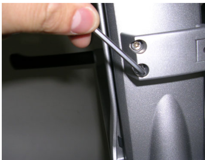
Figure 8-125 Removing the Cable Holder Bracket from the Support Arm
