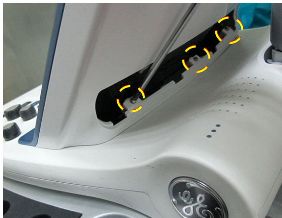
Figure 8-37 Removing the Rear Cover (Base) Securing Screws
