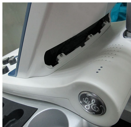
Figure 8-35 Removing the Touch Screen Service Cover
