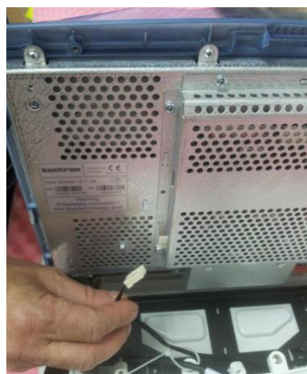
Figure 8-47 Routing and Connecting the Touch Screen Cables
