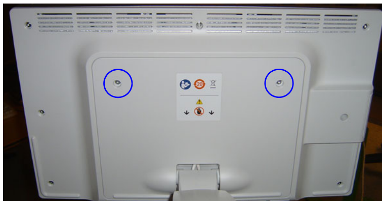
Figure 8-32 Monitor Rear Cover's fixing screws
