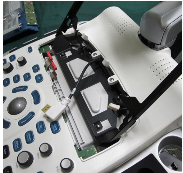
Figure 8-45 Removing the Touch Screen
