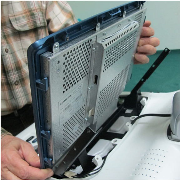
Figure 8-45 Removing the Touch Screen
