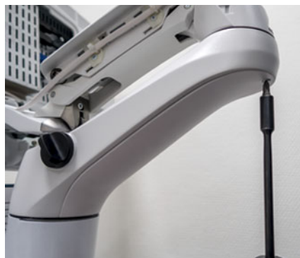
Figure 8-91 Remove the Lower Service Cover
