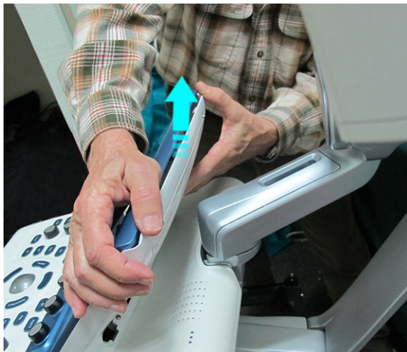
Figure 8-39 Removing the Touch Screen Rear Cover
