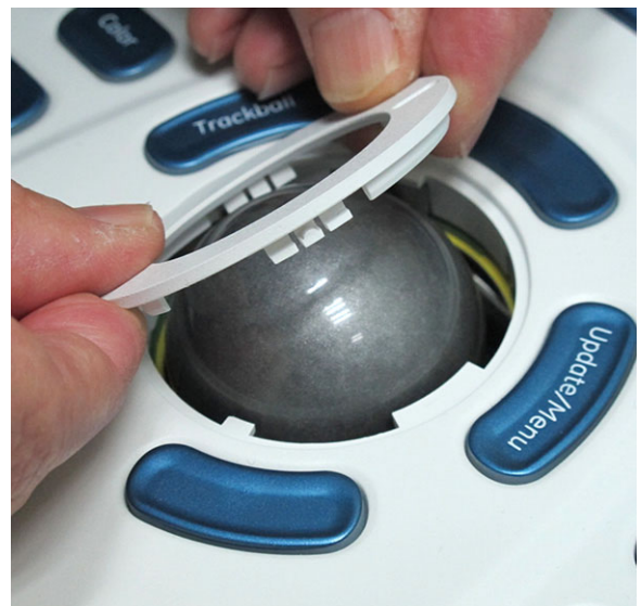
Figure 8-64 Removing the Mechanical Trackball Ring
