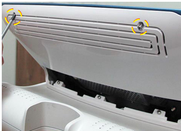
Figure 8-38 Removing the Rear Cover (Top) Securing Screws
