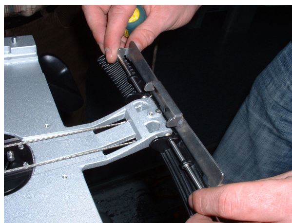
Figure 8-98 Protective Metal Plate Rotated 90 Degrees
