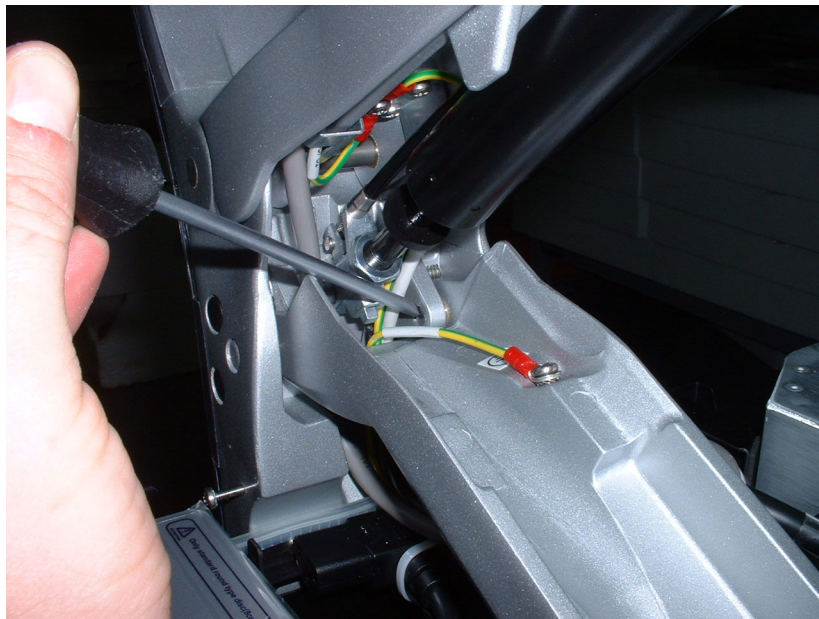
Figure 8-107 Removing Securing Pin and Disconnecting Ground Lead
