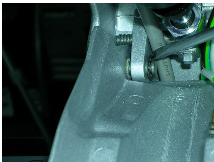
Figure 8-106 Removing Left Securing Clip from Securing Pin
