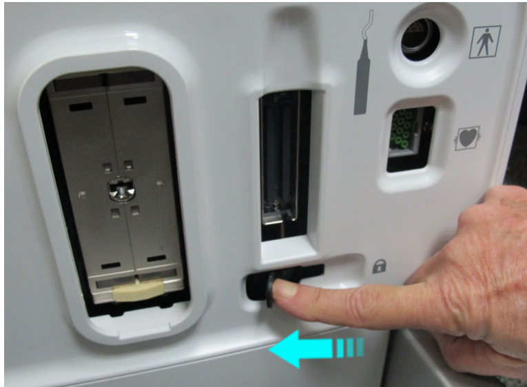
Figure 8-11 RS Probe Connector Lock - OPEN
