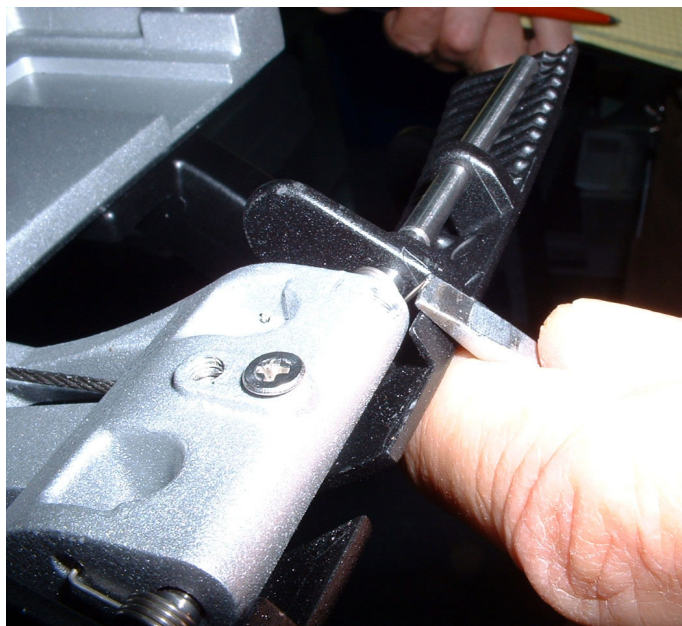
Figure 8-100 Releasing Spring that Presses on the Handle
