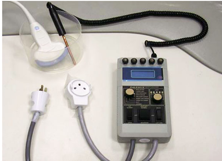
Figure 10-5 Test Set Up with Electrical Safety Analyzer
