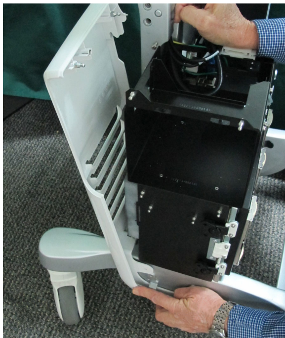
Figure 8-19 Removing the Right Rear Cover
