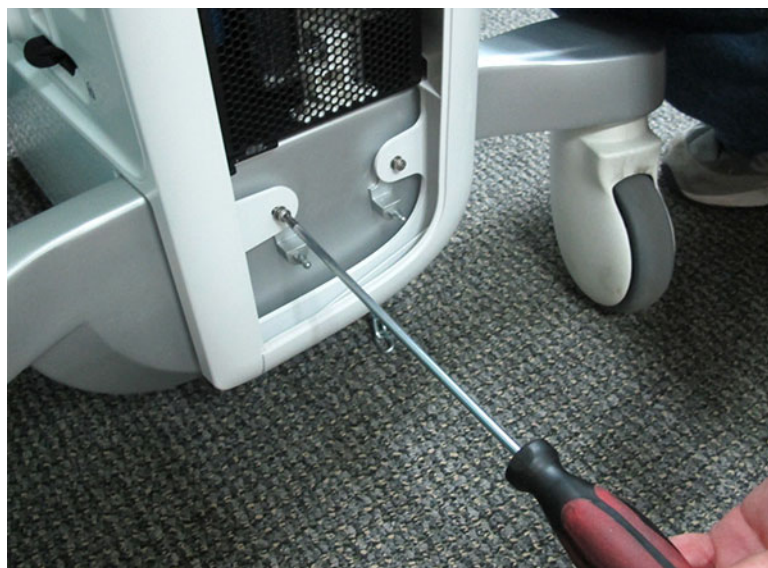
Figure 8-13 Removing Screw from Front Cover Securing Tab
