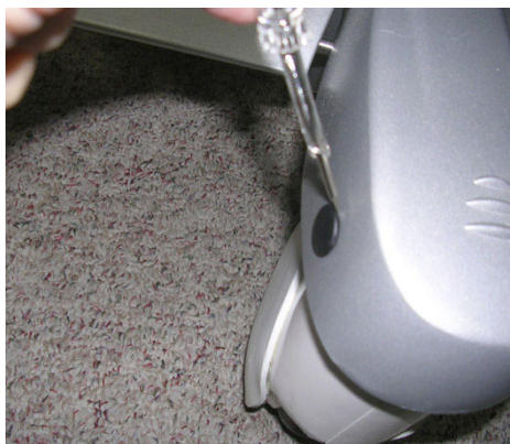
Figure 8-133 Removing the Screw Cap
