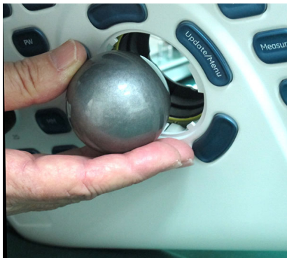
Figure 8-65 Removing the Mechanical Trackball
