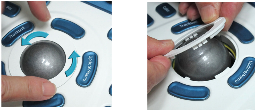
Figure 4-14 Removing Top Locking Plate and Rubber Dust Filter Ring
