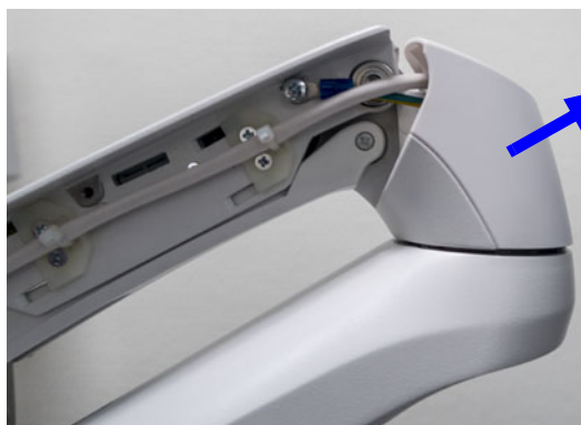
Figure 8-90 Remove the Vertical Service Cover
