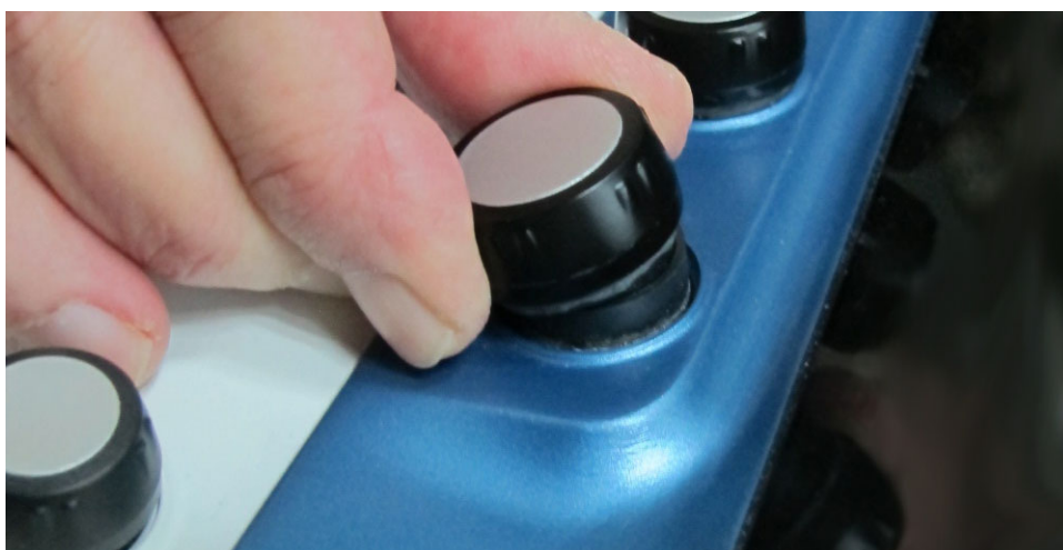
Figure 8-68 Removing a Rotary Knob
