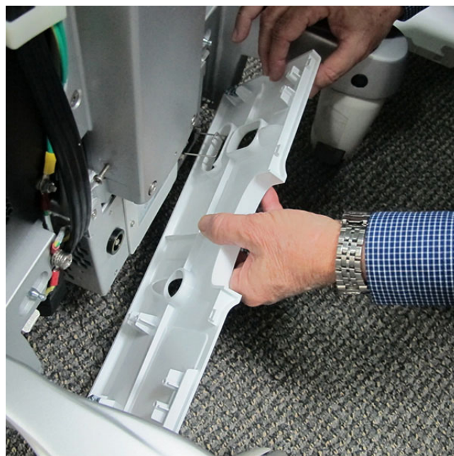
Figure 8-30 Removing the AC Distribution Box Cover
