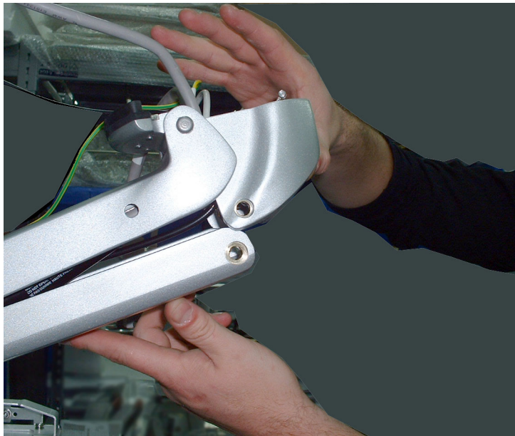
Figure 8-109 Raising Lower Arm to Reconnect with Upper Arm (Console not shown)
