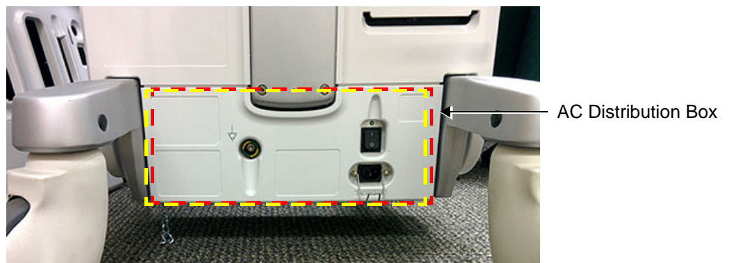
Figure 8-80 AC Distribution Box Located at Rear of System
