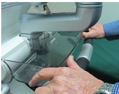
Figure 8-25 Installing the OPIO Basket
