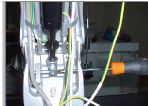
Figure 8-112 Tapping out the Lower Support Pin using a Punch
