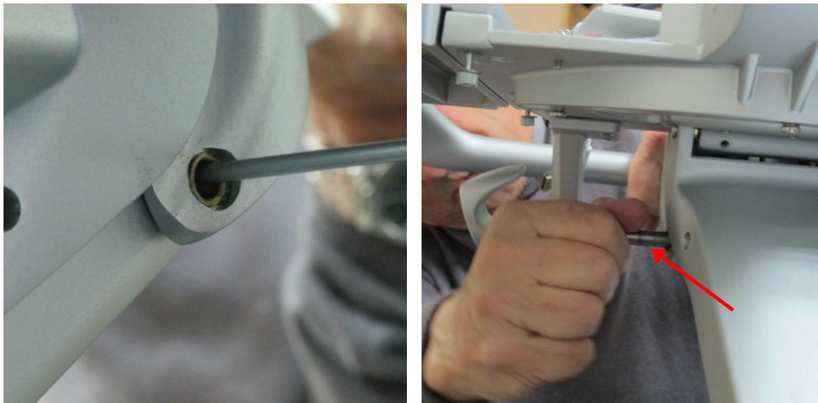
Figure 8-104 Remove Securing Pin
