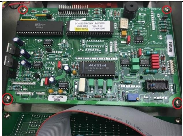
9. Use a #1 Phillip screwdriver to remove the screws on the display board
