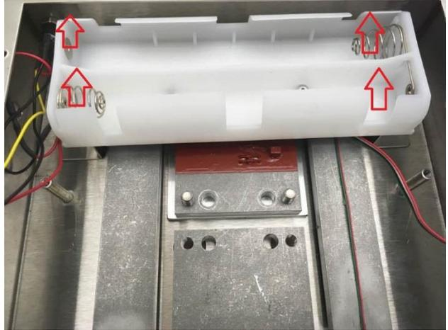
17. Remove the two remaining nuts on the load beam using a 10mm socket
