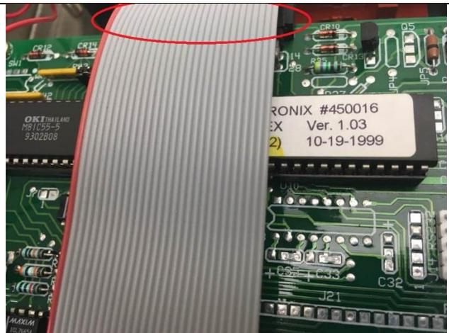
7. Disconnect the J1 Power connector from the board
