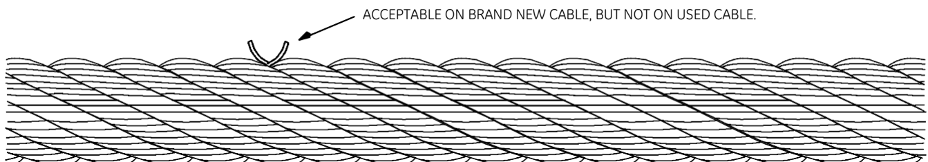
ILLUSTRATION A-8 SINGLE CROWN WIRE BREAK
