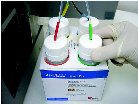
**Figure 4.2** Place reagent pack inside the Vi-CELL XR reagent compartment
