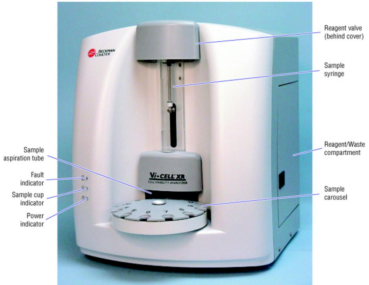
**Figure 2.3 Right side of the Vi-CELL XR showing reagent compartment**
