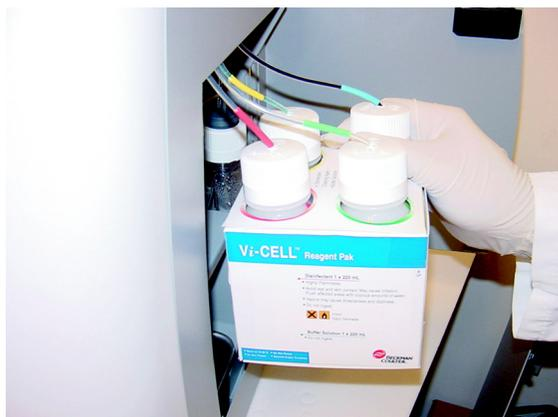
**Figure 4.3 Attach waste line to waste container and place inside the Vi-CELL XR**
