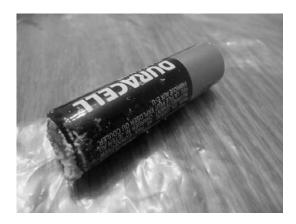
This picture shows a leaking battery.
