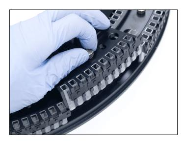
**12** Place the cuvette wedge upside down on the protected surface to remove the cuvettes. Use your finger or the reverse end of a cotton-tipped applicator stick to gently push the cuvettes out of the wedge. Remove all 330 cuvettes.
