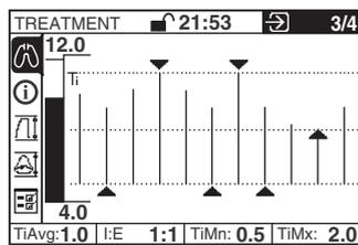
Treatment screen 3 displays the live Ti bar history (Ti Graph). The far left Ti bar (to the right of the Pressure bar) is constantly active, showing the current breath (this Ti bar also appears on other screens during treatment). The Ti graph displays the animated Ti bar history for 10 breaths before the screen refreshes. The far right bar always shows the most recent breath.
