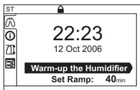
If using a HumidAire 2i with the device, you can use the Warm-Up feature to pre-heat the water in the humidifier prior to starting treatment. The HumidAire 2i will be automatically detected when the device is turned on and the Patient Standby screen provides the option to start warming the humidifier.
