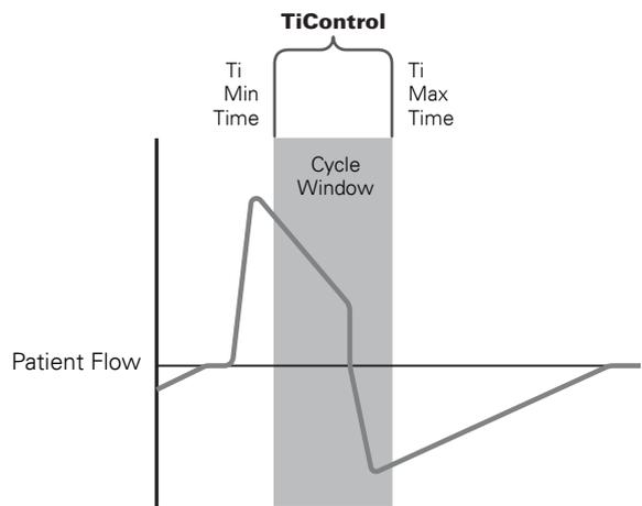
Figure 8: TiControl (Ti Min and Ti Max Time Parameters) sets the Cycle Window
