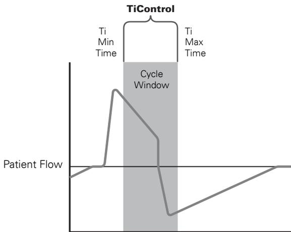
Figure 2: TiControl (Ti Min and Ti Max Time Parameters) sets the Cycle Window
