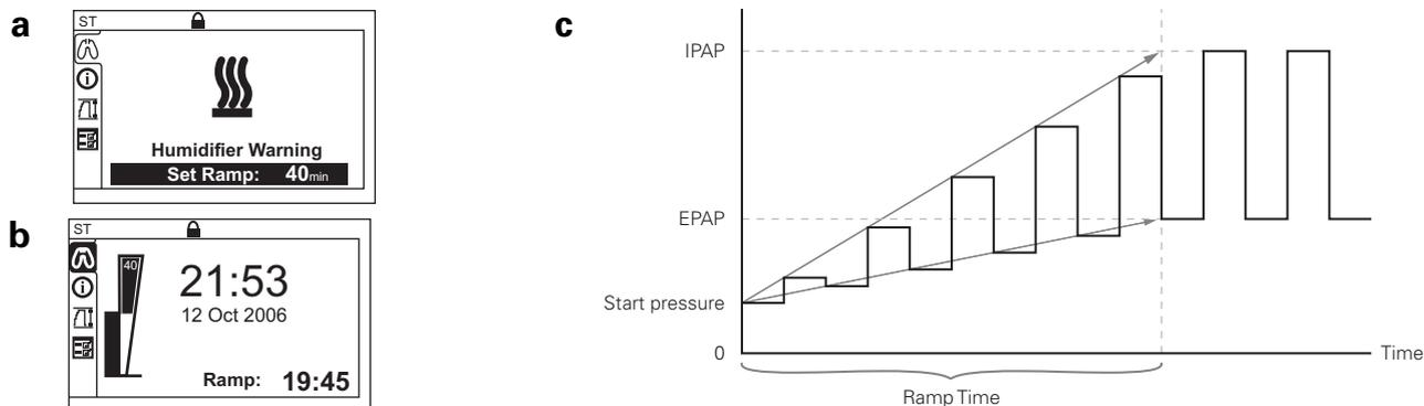
Figure 5: (a) Patient Standby screen with Max Ramp set; (b) Therapy running with Ramp; (c) Ramp in bilevel mode.
