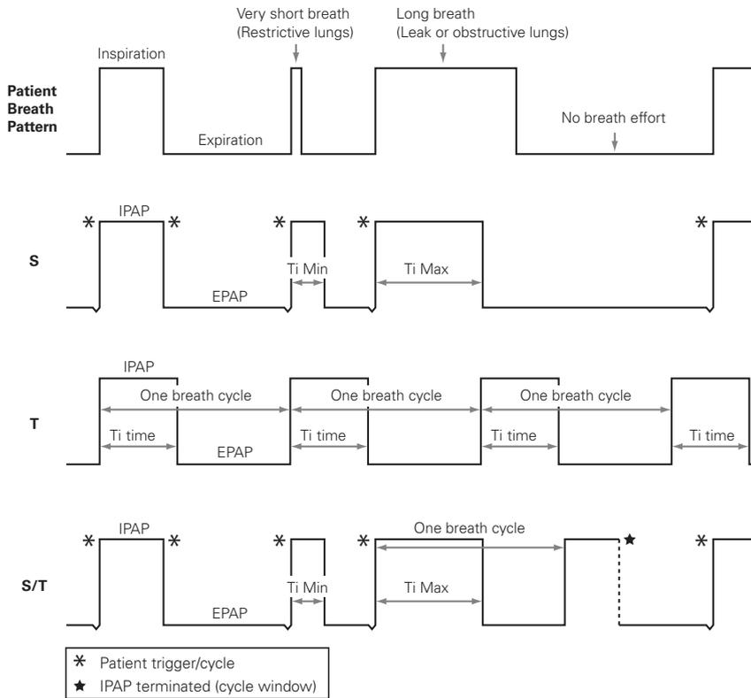
Figure 3: VPAP III ST-A with QuickNav modes
