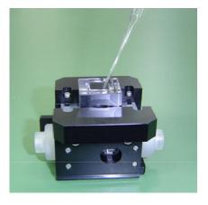
**6** Remove any bubbles and/or foam, and insert the cell cap. Ensure that there are no bubbles or foam below the Daifron plunger.
