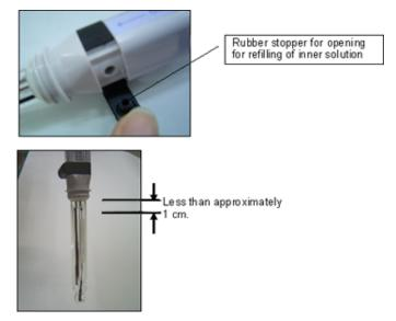
**4** Wash the tip of the electrode with purified water, and wipe with a soft cloth.
