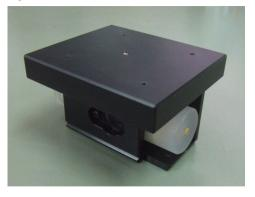
Figure 4.48 Disposable Cell for Zeta Potential Components
