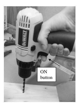
Continue holding the ON button. Gently push the drill bit through the material. Release the ON button once the drill bit goes through the other end.
