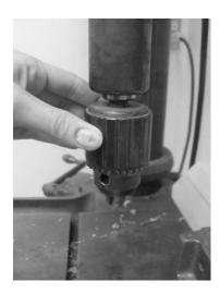
Insert the drill bit into the chuck. Twist the chuck to the right to tighten it.
