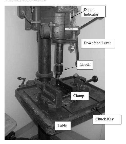
A clamp or vise holds the material firmly. A clamp prevents slipping. There are many types of clamps. Use a clamp to secure the drilling material.
