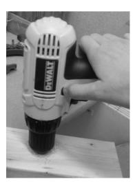
Press the ON button. Slowly lift the drill away from the material. Release the ON button once the drill bit is out of the material.
