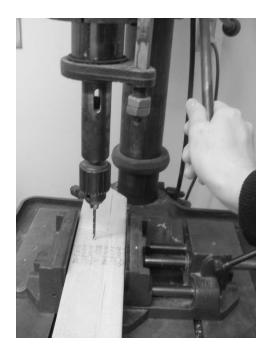
Lower the drill bit close to the material. Turn the machine on. Use cutting fluid in appropriate quantities. Use the downfeed lever to lower the drill bit through the material. Do not push too hard. You will feel the drill bit go through the other side. Slowly and gently lift the downfeed lever up. One the drill bit is out of the material, turn the machine off.
