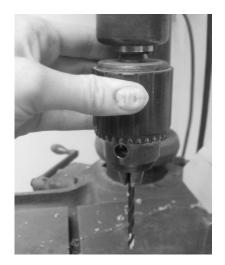
Use the chuck key to tighten the chuck completely. Insert the chuck key into the hole on the chuck. Rotate the chuck key to the right.
