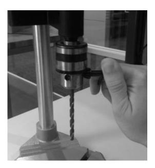
Verify that the drill bit is secure. The threaded section of the drill bit should be completely visible. Verify that the drill bit is in the chuck straight.
