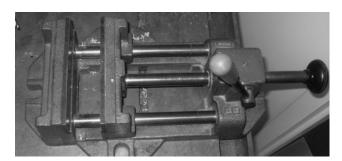
Place the material in the clamp. Close the clamp. Verify that the clamp is secure.
