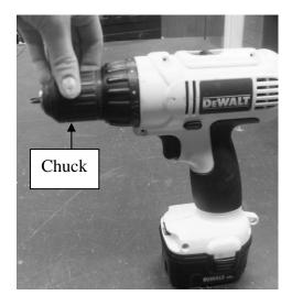
Insert the drill bit. Twist the chuck to the right to tighten it.
