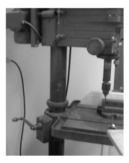
Position the material and clamp under the drill bit. Use the downfeed lever to lower the drill bit. Do not turn the machine on yet. Verify that the drill bit will hit the desired spot.
