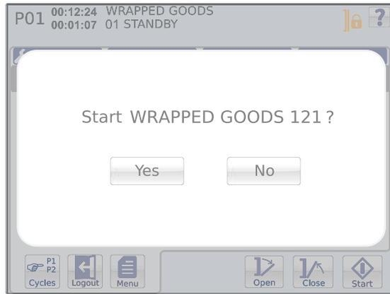
The window remains on the screen until a selection is made by pressing the desired button.
