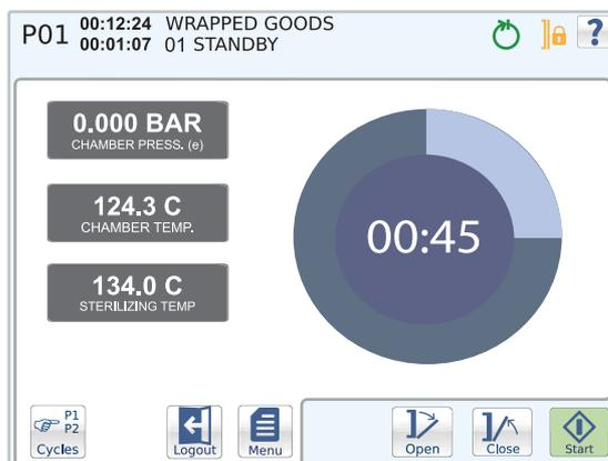
The pie chart graphically displays the time remaining for the cycle. The circle diagram also displays the time remaining in digit form.
