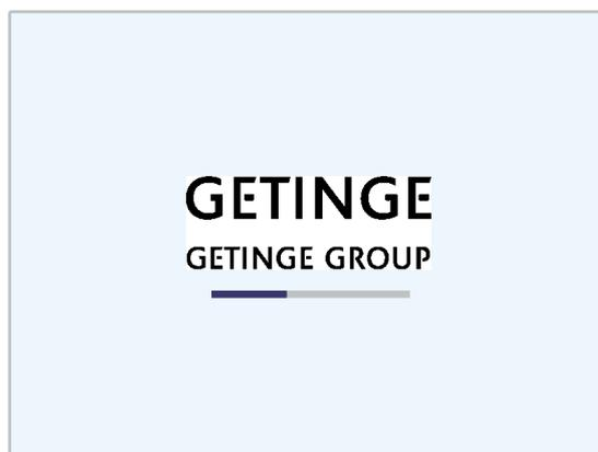
In case of communication errors between the panel and the operating system, the blue bar travels back and forth. There is no communication with the operating system as long as this screen displays and no command can be sent to the operating system.
