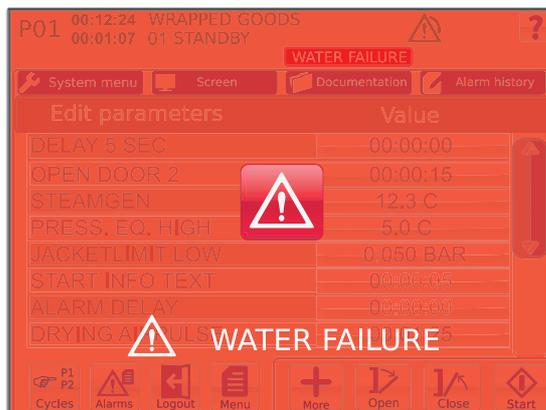
In the event of an alarm, the current alarm displays as a pop-up window on the screen and an alarm sounds. For alarm management, see the "Alarm" section in the chapter *Operation* of the USER MANUAL.
