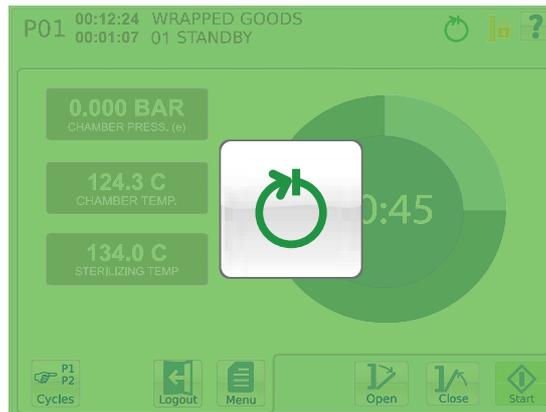
The window remains on the screen until the acknowledgement button is pressed or the door is opened automatically.
