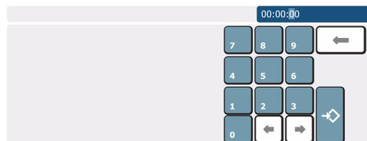
To edit the time, mark the number you wish to edit using the arrow keys at the bottom. Press the desired number. To save the entry, press **Save** at the bottom right.
