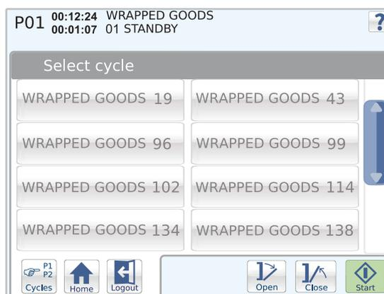
To select a cycle, press the desired cycle. The previous screen is displayed again.
