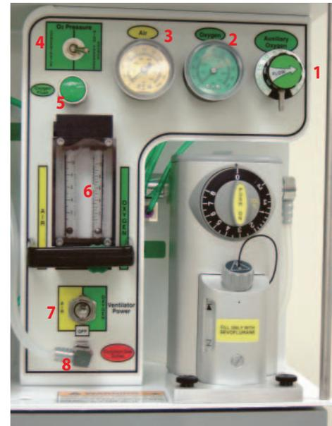
**1. Auxiliary O2 Flow Selector:** Designed to allow the operator to supply oxygen to a patient pre and post-op with small bore tubing for a nasal cannula or disposable oxygen mask. The selector knob will allow the operator to provide oxygen flow at 2,4,6,10 and 15 liters per minute.
