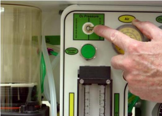
**NOTE:** Use of the Air Compressor is the preferred ventilator gas power source in order to conserve cylinder oxygen sources.
