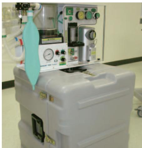
**7. Attach small O2 cylinder mount to box back.**
