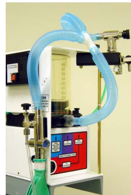
**WARNING:** Scavenger system should always be mounted in order to keep debris from entering the bellows outlet port.
