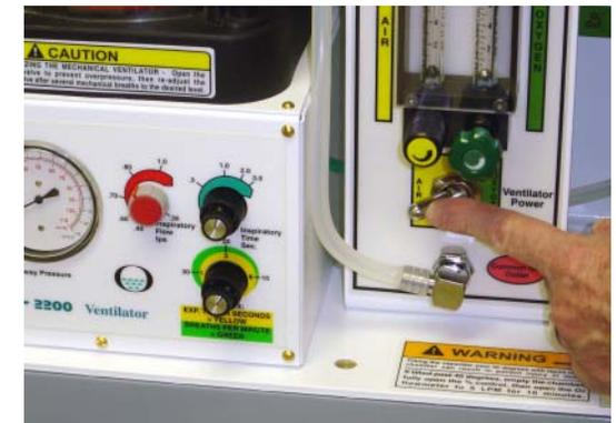
**1. Power Source:** Air or oxygen delivered to the gas manifold at 40-70 PSI, 50 PSI Optimal.
