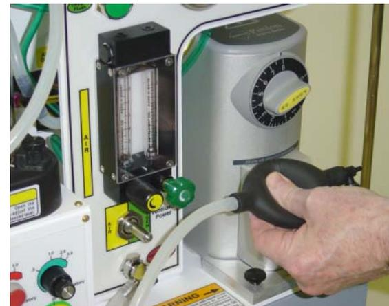
A. Adjust flow of Oxygen and Air through their full range, checking for smooth operation of floats and undamaged flowtubes.
