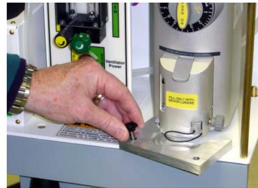
**B.** Remove the two holding knobs and spacer plate from the back plate located on the backside of the frame behind the vaporizer.
