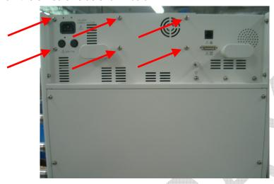
2 Take out the power box after disconnecting the cables from the power conversion board marked in the picture.
