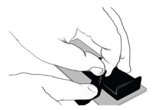
5. Using solid core wire, solder the negative lead on the battery holder to the resistor.
