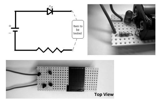
8. You should now have two wires extending from the perfboard. Strip the ends of the wires. Solder an alligator clip to each wire. The clips are terminals that connect to the connections you will test.
