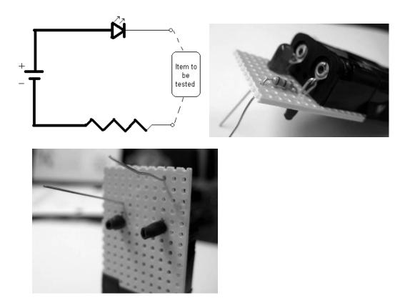
7. Prepare two lengths of stranded wire for the test leads. Cut two stranded wires at least 15cm long. Solder one wire to the negative end of the LED. This is the positive lead. Solder the other wire to the free end of the resistor. This is the negative lead.
