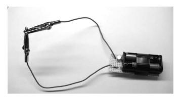
10. You may use electrical tape or heat shrink tubing to insulate the alligator clips. Shrink any remaining heat shrink tubing to cover the connections. Use epoxy to attach the battery holder to the perfboard.
