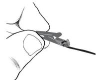
9. Clip the test leads together. This creates a closed circuit. The LED should light if the continuity tester is assembled correctly. If the LED does not light, check your connections.
