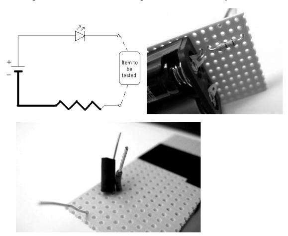
6. Using solid core wire, solder the positive end of the LED to the positive lead of the battery holder. Remember, the positive end of the LED is the long lead.
