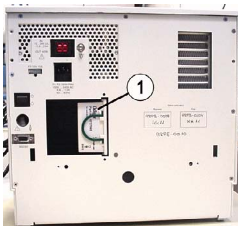
Fig. 24 Savina rear (filter cover removed); fitting location of microfilter
