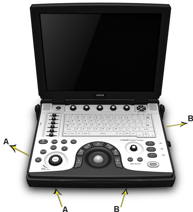
Figure 5-2. Air Flow Inside the System
