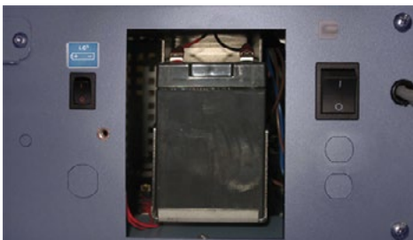
Monitoring system backup battery (supplies power to optional Access Control system).
