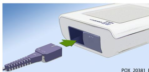
2. Connect the OxiMax™ DS-100A sensor to the DEC-4 cable, then to a finger.
