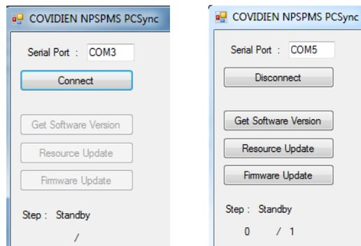
7. Complete the connection between the monitoring system and the PCSync™\* utility by using the PC's Device Manager to determine the serial port number for the USB to UART Bridge.
