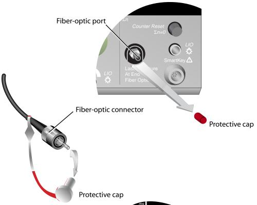
Carefully insert and fingertighten the connector into the console fiber-optic port until secure.
