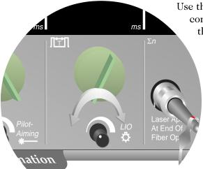
Use the illumination brightness control on the console to adjust the intensity of the white illumination beam.
