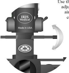
Use the aiming beam/treatment beam adjustment control to position the red aiming beam within the field of view. The console delivers the treatment beam to the site illuminated.
