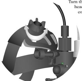
Turn the knob at the top of the headpiece until the headband is comfortably positioned.
