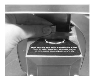
Verify calibration: Locate an object whose precise weight is known and within the range of the scale. If you do not have an object of known weight, you must create one. Use a syringe or graduated cylinder to measure a known volume of water. Water weighs one gram for each milliliter. So, if you need a weight of 20 grams, measure 20 milliliters of water.
