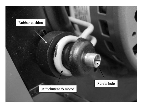
Evaluate the rubber cushions. Replace rubber cushions that are cracked, hardened, or broken. If you cannot find replacement rubber cushions, cut a similar rubber piece out of surgical tubing or bike tubing.
