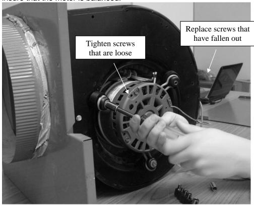
**Tightening the Screws:** In order to tighten the screws evenly, tighten the screws sequentially and in a pattern. Following the numbering pattern, tighten the first screw a few turns. Next, tighten the opposite screw a few turns. Continue the pattern of tightening a little until all the screws are evenly tightened. Do not tighten one screw fully before tightening the other screws.
