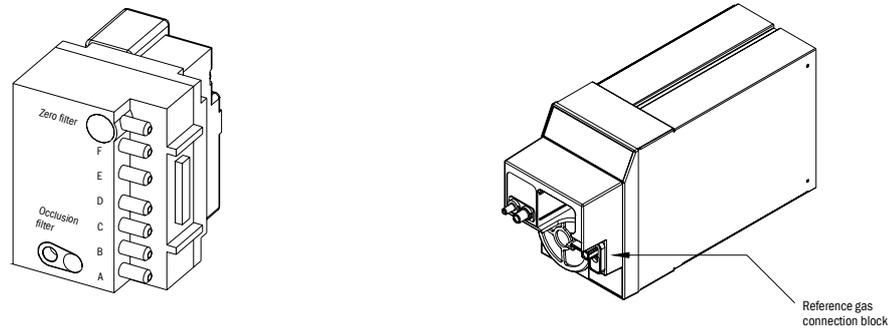
**Figure 16 Pneumatic unit and reference gas connection block**
