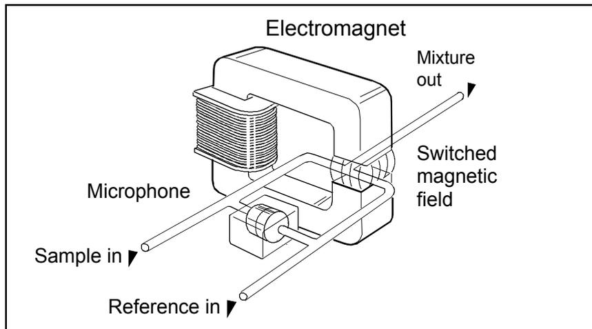
**Figure 4** O<sub>2</sub> measurement principle
