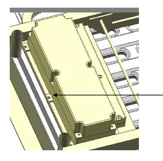
Top of the control box shall be assembled with bed frame by bolts.
