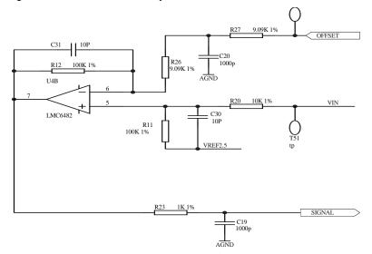
Fig 2-5 Voltage Shift Circuit
