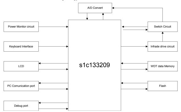
Fig 2-1 DPM1 Pulse oximeter Block Diagram
