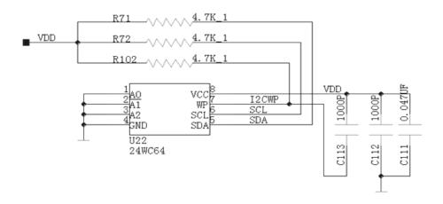
Fig 2-3 Data Storage Circuit
