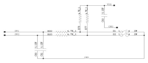
Fig 2-9 Button Circuit
