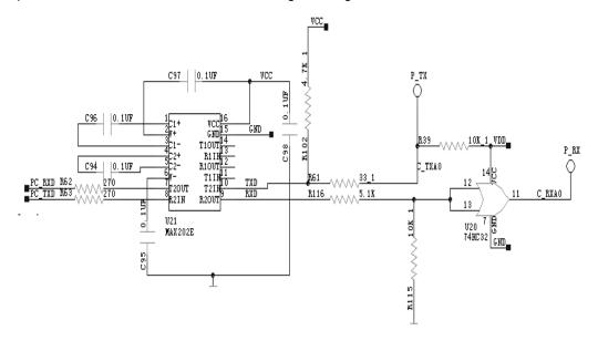
Fig 2-8 Serial Signal Voltage Level Conversion Circuit
