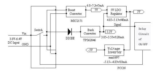
Fig 2-10 Power Supply Circuit Block Diagram
