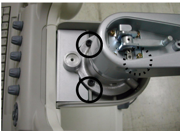
Figure 8-31 Separating the neck pipe
