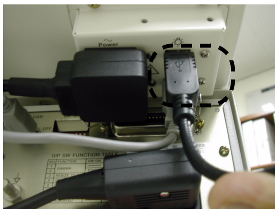
Figure 8-323 Additional Task Lamp Installation
