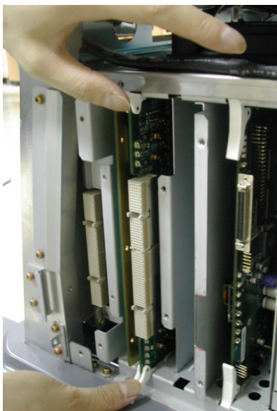
Figure 8-110 Eject the CL1TRX(BL1TRX) Board
