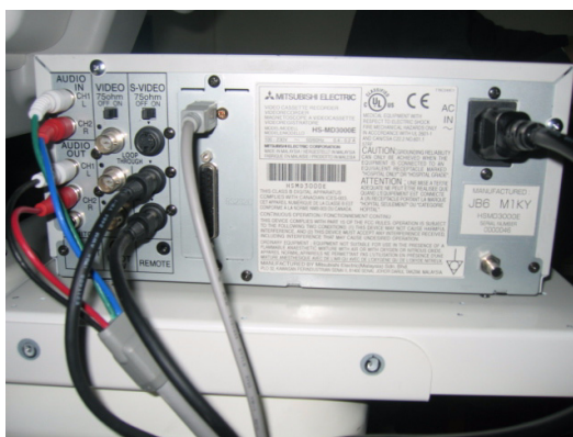
Figure 8-306 Printer VCR DVD Fixture Top installation
