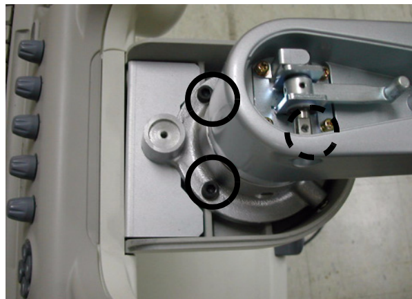
Figure 8-45 Assembling the arm neck pipe
