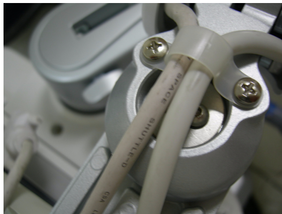
Figure 8-54 Assembling the Cable clamp
