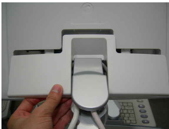
Figure 8-16 Removing the LCD cable cover
