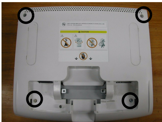
Figure 8-8 Removing the LCD rear cover
