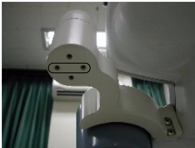
Figure 8-246 Endo Probe Holder Installation
