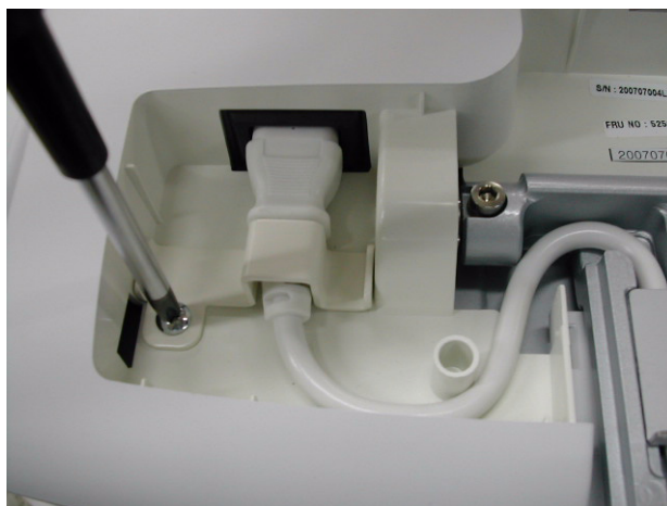
Figure 8-17 Removing the power cord bracket
