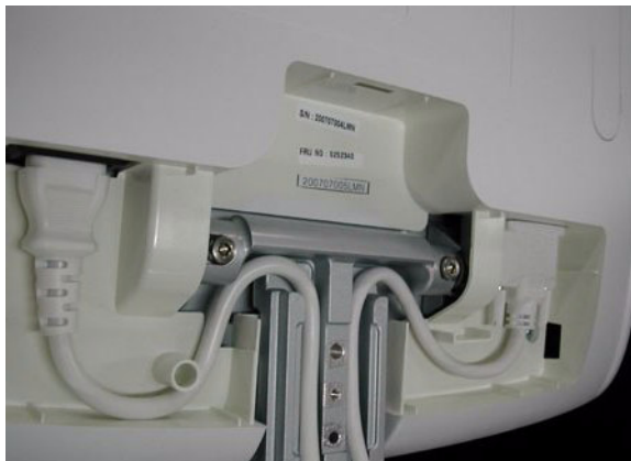
Figure 8-52 Placing the Cables
