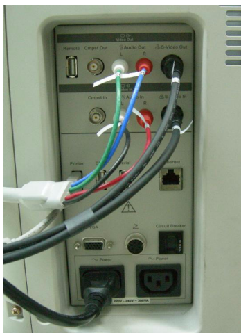
Figure 8-316 Printer VCR DVD Fixture Top installation (LQ MD800)
