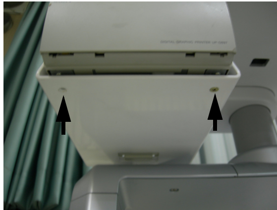
Figure 8-261 BW Printer Fixture Keyboard installation
