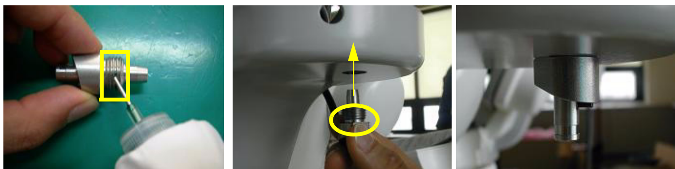
Figure 8-37 Screwing the spring holder Assy
