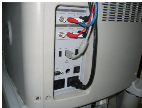
Figure 8-307 Printer VCR DVD Fixture Top installation
