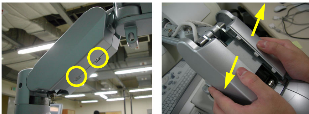
Figure 8-22 Removing the Arm cover L & Arm cover R
