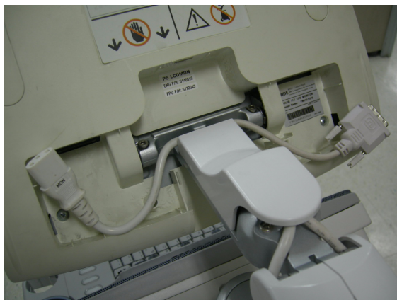
Figure 8-18 Disconnecting power cable and DVI cable
