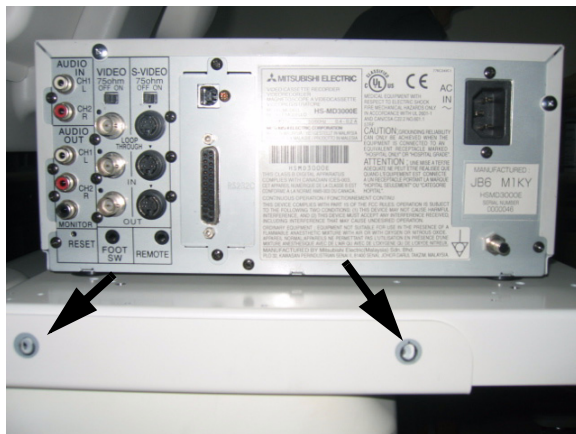
Figure 8-305 Printer VCR DVD Fixture Top installation
