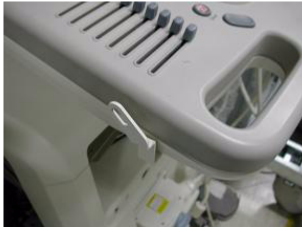
Figure 8-249 installation of Microphone
