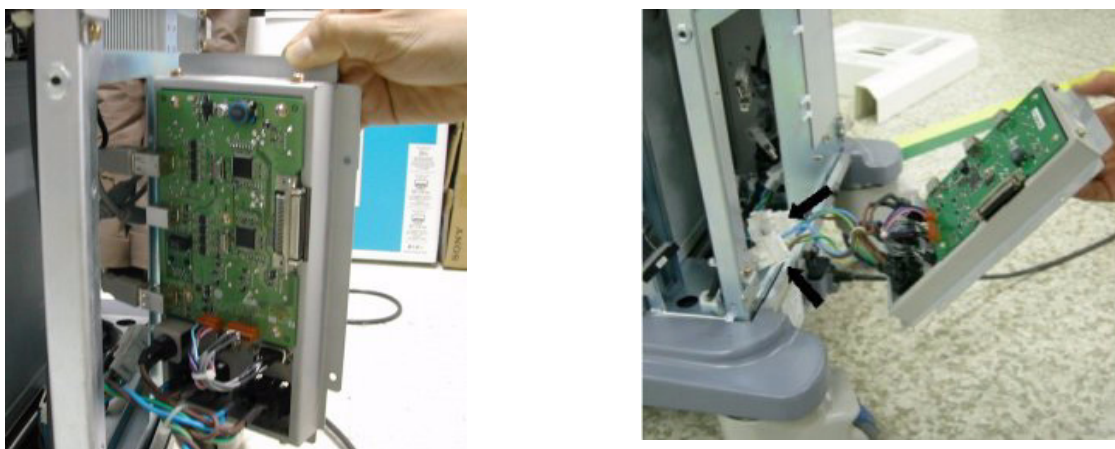
Figure 8-142 Open Rear Panel
