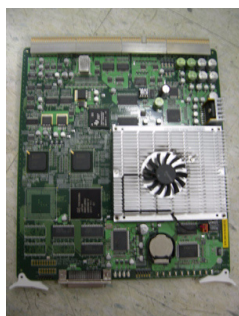
(a) Cooling Fan on SYSCOMPM(SYSCONCM)
