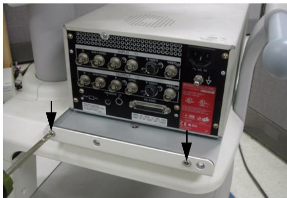
Figure 8-282 Printer VCR DVD Fixture installation top
