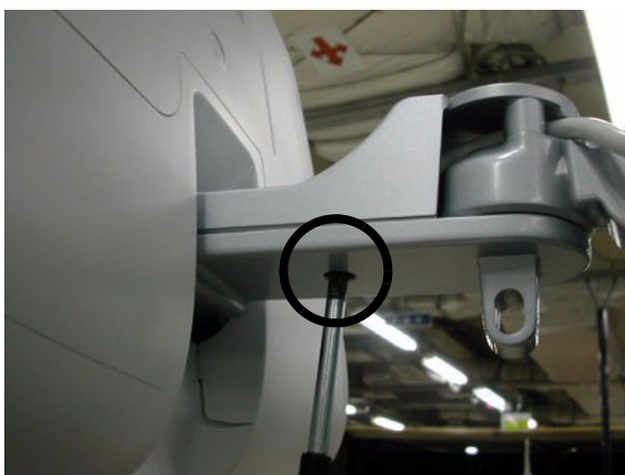
Figure 8-19 Removing the Fold cover
