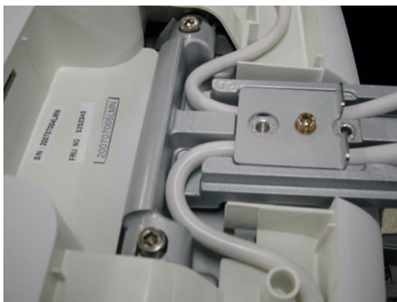
Figure 8-53 Assembling the Cable bracket
