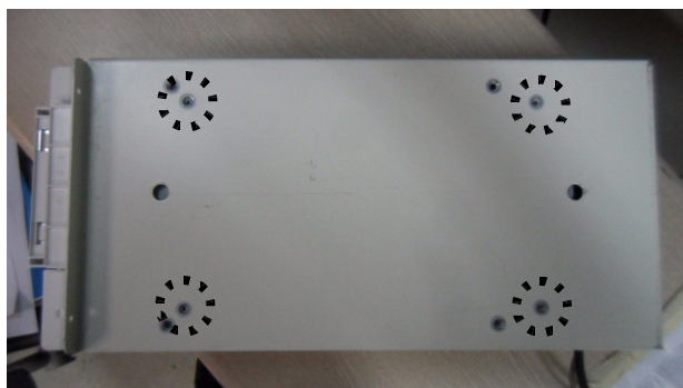
Figure 8-288 Color Printer Fixture Top Installation
