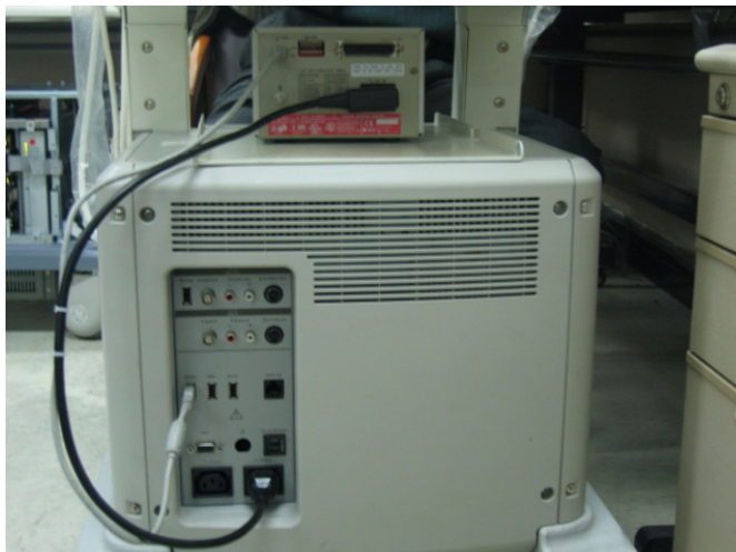
Figure 8-266 BW Printer Fixture Middle installation
