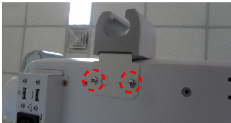
Figure 8-339 MTZ PROBE HOLDER Installation
