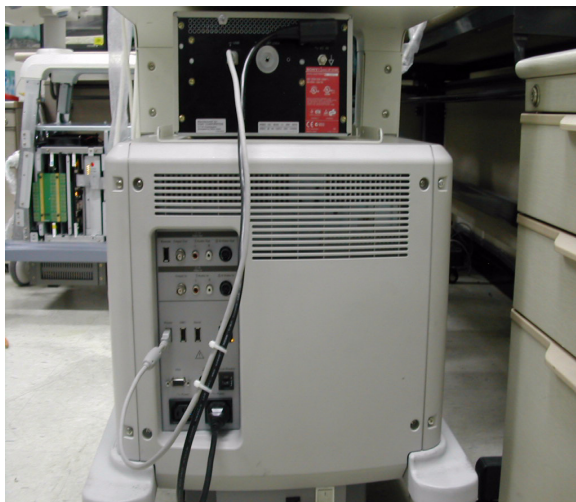
Figure 8-271 Color Printer Fixture Middle installation
