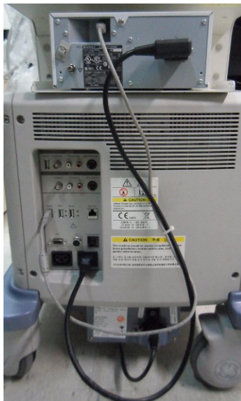
Figure 8-276 Color Printer Fixture Middle installation
