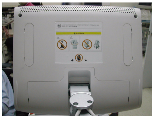
Figure 6-5 Putting the label on the rear of the LCD monitor
