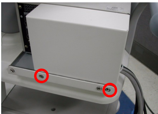
Figure 8-283 Printer VCR DVD Fixture installation top
