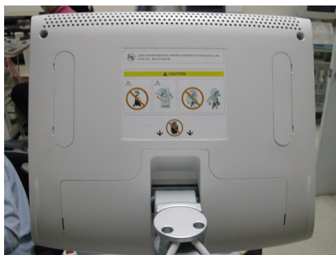
Figure 8-3 Putting the label on the rear of the LCD monitor
