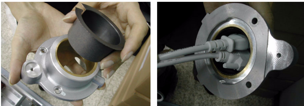
Figure 8-41 Inserting the oilless bush
