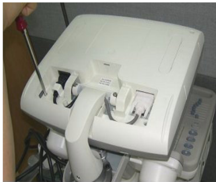
Figure 8-15 Disassemble Monitor from STD arm
