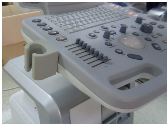
Figure 8-340 MTZ PROBE HOLDER Installation
