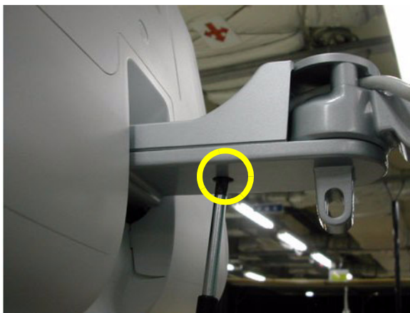
Figure 8-62 Assembling the Fold Cover
