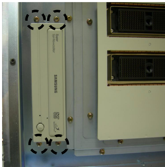
Figure 8-135 Unscrew 4screws and remove the DVD Assy
