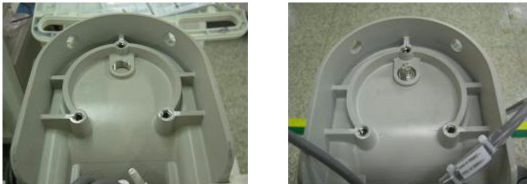
Figure 8-38 Screwing the spring holder Assy
