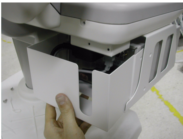
Figure 8-327 Additional Task Lamp Installation
