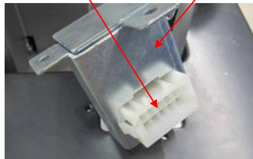
The socket of spring cable Fixing bracket of spring cable
