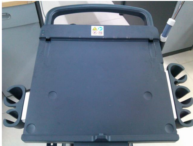
Figure 9-4 Installation for holders on right and left sides
