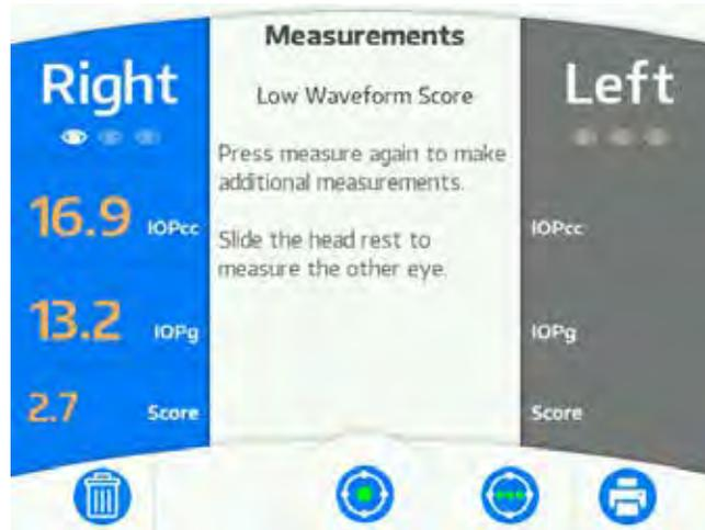
**Note:** It is possible that post refractive surgery eyes, eyes with corneal pathologies, and glaucomatous eyes will produce consistently low measurement scores. The IOP values based on the highest obtainable scores should be considered reliable.
