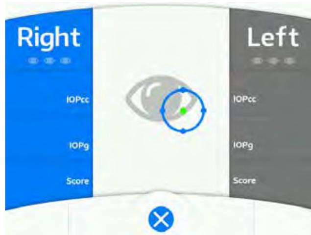
During the alignment and measurement process, the Operator Display will show the position of the airtube with respect to the center of the patient's cornea. As the positioning system aligns to the apex of the eye, the measuring icon will move to the middle of the screen and align over the center alignment mark (+). Once the positioning system is aligned the air "puff" or "puffs" are delivered to the eye and the IOP measurement is automatically displayed.
