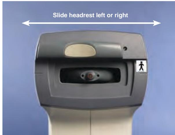
The Reichert 7CR features a left/right sliding forehead rest that enables the instrument to automatically determine which eye is being measured. It must be positioned completely to one side or to the other in order to take a measurement. Position the forehead rest to the desired position before beginning the measurement process.
