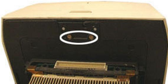
5. Push the reaction module lid open. Notice that the latch (dark plastic) is no longer attached. Remove your samples from the block.
