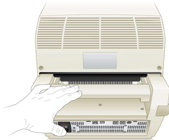
2. Carefully lift the optical reaction module out of the bay using the handle indents on each side.
