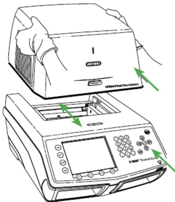
3. Pull up the locking bar until it is flush with the sides of the module bay. This action moves the module forward, locking it into place.
