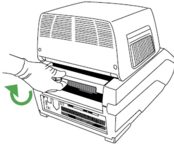
4. Check that the module is completely and evenly seated in the C1000 Dx thermal cycler base. There should be no extra space between the module and the base.
